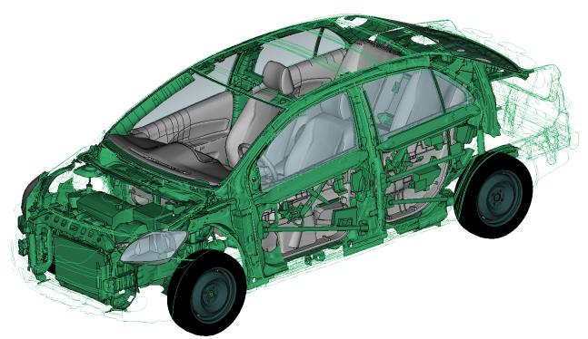
Figure 4. The FE-model also contains representations of the engine, instrument panel, seats etc.
