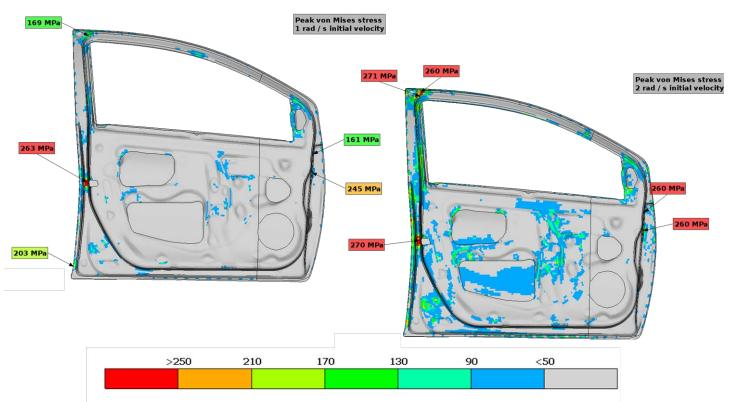
Figure 10. Stress results from the door slam load cases. The left image shows the peak von Mises stress for 1/rad initial rotational velocity, and the right image shows the corresponding results for 2 rad/s initial velocity.
