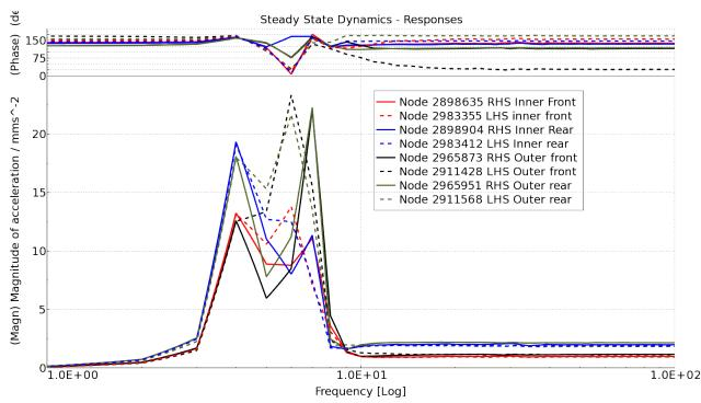
Figure 12. Acceleration responses (amplitudes in the lower image and phase in the upper image) in the seat attachment points as a function of frequency.
