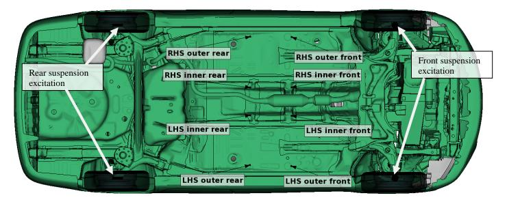
Figure 11. Load case definition for the steady state dynamics load case. The responses were evaluated at the attachment points of the front seats. The vehicle was excited by Z-forces applied at the suspension, corresponding to 50 % of the static load. The left and right-side excitations were completely out-of-phase, while the front and rear suspension excitations have opposite signs.
