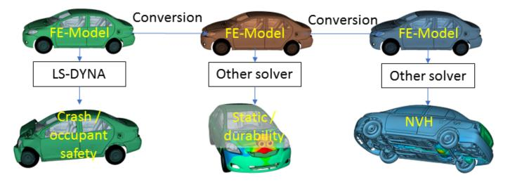
Figure 1. Outline of traditional work flow for FE-analyses in the automotive industry.
