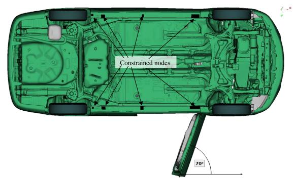
Figure 7. Constrained nodes for the door sag load case. The suspension was constrained at the hubs. The door opening angle was 70°.
