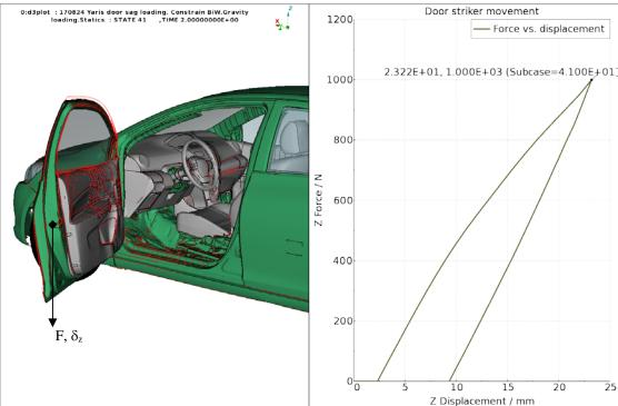
Figure 8. Results from the door sag analysis. The left image shows the maximum deformation, with an overlay of the original configuration shown as red feature lines. Also, the load application location is indicated. The right image shows the force – displacement curve for the door sag load case.
