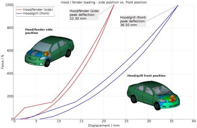
Figure 9. Results from the hood / fender load cases.
