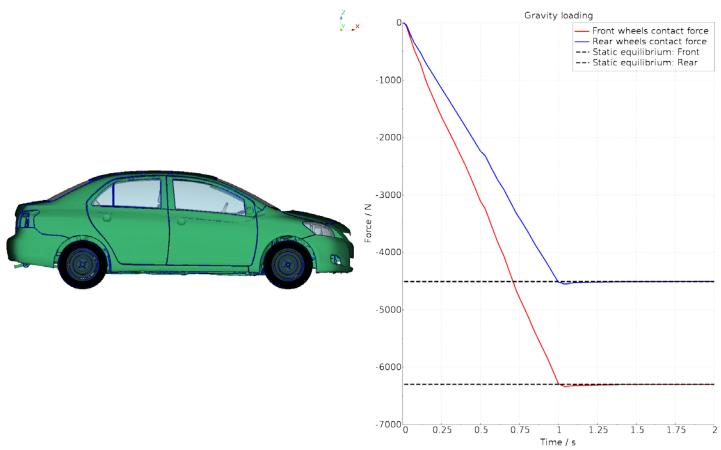
Figure 6. Gravity loading results. The left image shows the final configuration, with an overlay of the initial configuration in blue feature lines. Only small deformations can be noted. The right image shows the force balance as a function of time.
