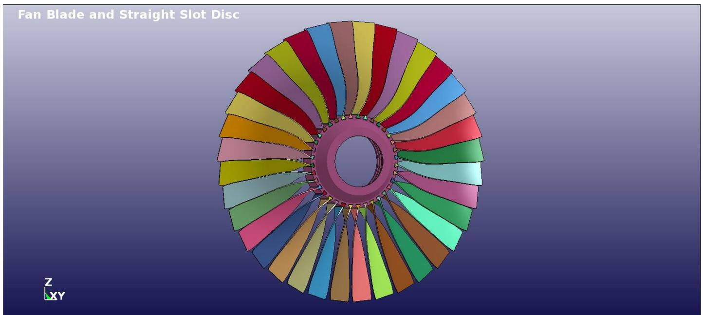
Instead of using the full model with 36 fan blades we can instead focus on just a single fan blade
