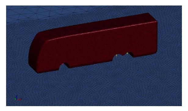
Figure 4: CFD surface mesh (LS-DYNA).
