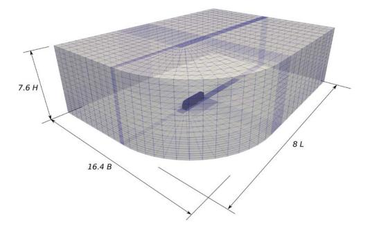
Figure 3: Configuration of the computational domain mesh (OpenFOAM).
