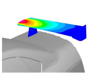
Figure 13 Maximum principal stress on spoiler during FSI simulation
