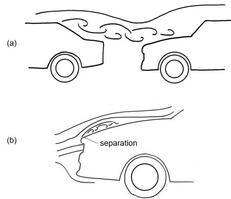
Figure 1 Extraneously induced excitation from the wake of a preceding car (a) and Instability induced excitation from separation at the front edge of a hood (b)
