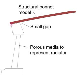
Figure 15 Close up of detail around the front of the 2D car model
