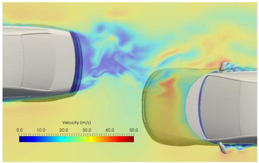
Figure 8 Flow field around the front of the following car
