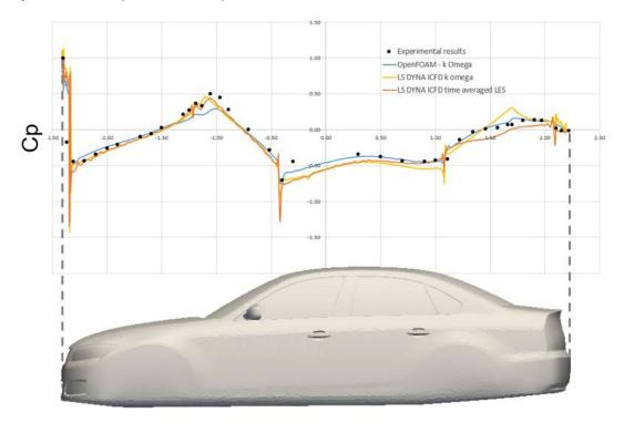
Figure 5 Pressure profile along the centreline of the DriveAer car
