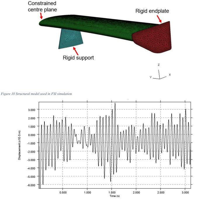
Figure 11 Time history of the vertical displacement of the end plate
