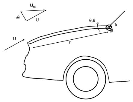
Figure 2 A hood mounted on a damped spring
