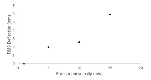
Figure 19 RMS deflection of the edge of the hood at a range of freestream velocity conditions
