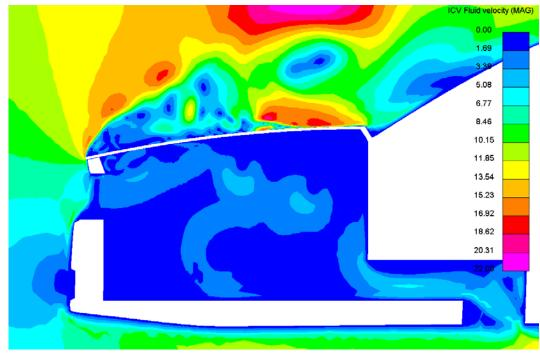
Figure 16 Velocity Contours from CFD simulation of sharpened hood profile
