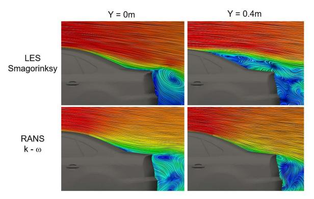
Figure 6 Velocity profiles around the rear window from the RANS and LES simulations
