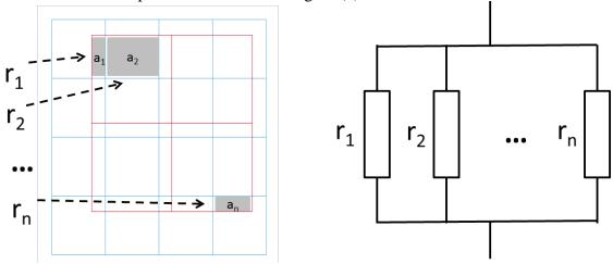
Figure 4 Illustration of contact resistance on the whole contact as a sum of n resistances in parallel
