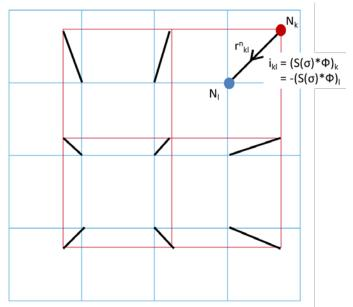
Figure 5 Illustration of the local node to node resistances used to connect the 2 parts using the contact resistances locally defined by the \*DEFINED\_FUNCTION
