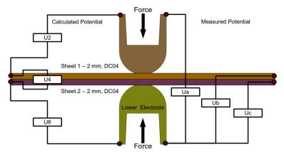
Figure 9 Experiment and location of measured and calculated potential differences
