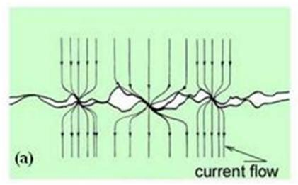
Figure 1 Illustration of the current flow at the contact of 2 materials at a microscopic level
