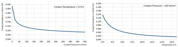
Figure 8 Example electrical contact resistance according Jonny-Kaars-Model
