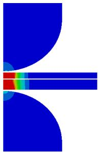
Figure 7 2D RSW model (Note: the Y axis is the symmetry axis)
