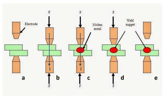
Figure 2 Steps of the resistive spot welding process: a) The 2 electrodes are placed on each side of the sheets to be welded. b) A force is applied on the 2 electrodes in order to create a pressure at the contact, and a current is sent through the electrodes
