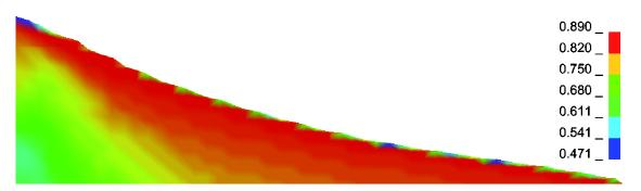
Fig. 9: Void ratio for the Hypoplastic UMAT soil material
