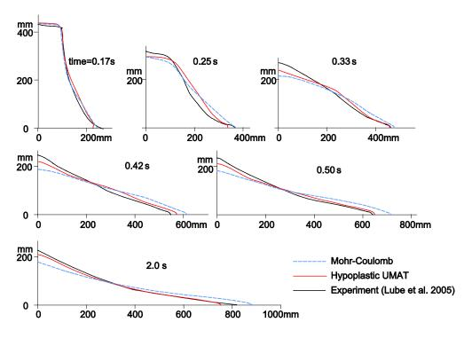
Fig. 8: Comparison of numerical results of sand column shape and distance with experimental measurements
