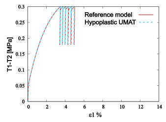
Figure 5 Deviatoric stress vs. axial strain for Triaxial compression test using the Hypoplastic UMAT
