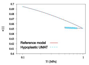
Figure 3 Void ratio vs. vertical stress curve for oedometric compression test using the Hypoplastic UMAT
