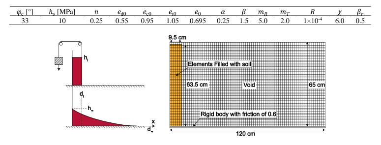
Fig. 6: a) Schematic view of the sand column problem b) initial numerical model configuration
