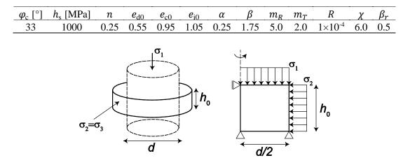
Figure 4 (a) Schematic of the triaxial test (left), FE-mesh and boundary conditions (right)
