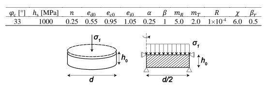
Table 5 Hypoplastic parameters of Hochstetten sand for Oedometer test [10]
