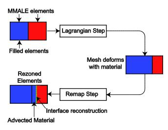
Fig. 1. Schematic diagram of MMALE sub-steps in one calculation cycle for one dimensional flow [2].
