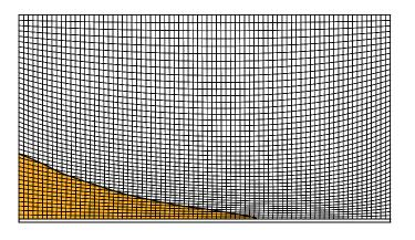
Fig. 7: Final numerical result of the sand shape using the Hypoplastic UMAT
