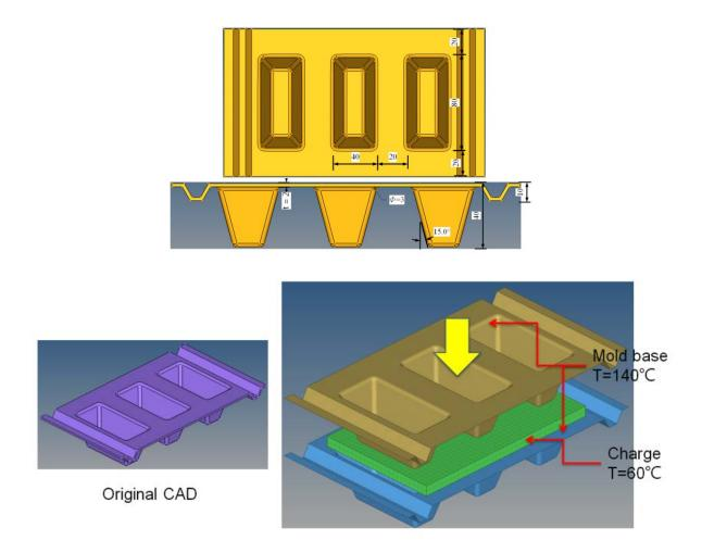
Figure 3. Compression molding model
