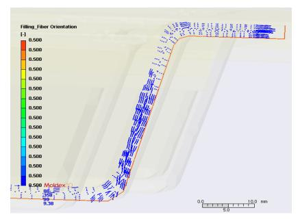
Figure 7. Initial fiber orientation in Moldex3D
