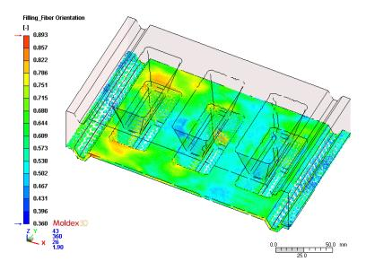
Figure 9. Fiber orientation at EOF
