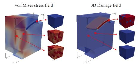
Figure 1 Illustration of a concurrent multiscale simulation based on RVE analysis and data-driven methods. The macroscopic material responses are driven by microscale RVE boundary value problem. The RVE package introduced in the paper will serve as the basis for the concurrent simulation.
