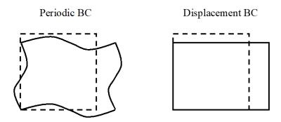
Figure 2 Illustrations of periodic and displacement BCs with the same macroscopic strain constraint on the RVE.
