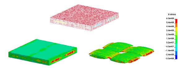
Figure 10 Simulation results of woven composites under uniaxial tension E11=0.01.
