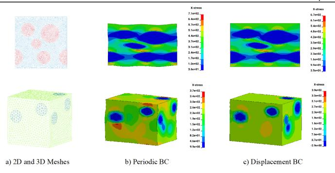
Figure 8 RVE analysis results under uniaxial tension (E11 = 0.4) for periodic and displacement BCs.
