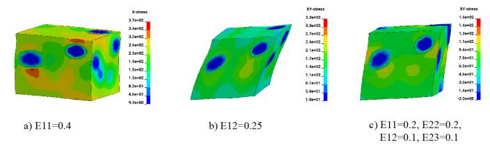
Figure 9 Simulation results under uniaxial, shear and mixed loading conditions
