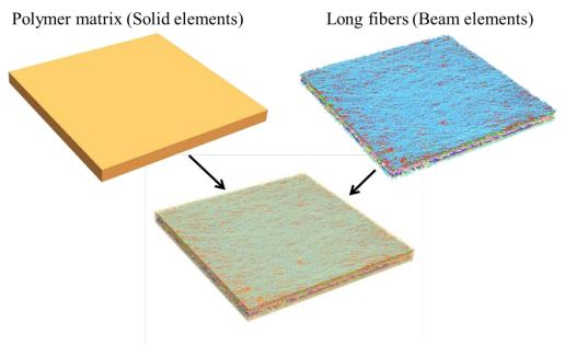
Figure 8: Polymer matrix by solid elements and Long fibers modelled by beam elements
