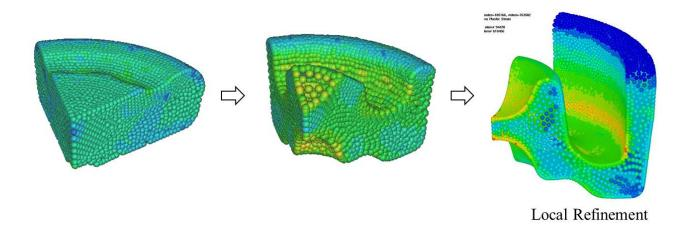
Figure 2: 3D forging simulation example using 3D adaptive EFG
