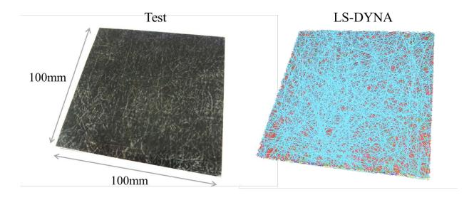
Figure 12: Long glass fiber reinforced thermoplastic sheet and LS-DYNA model
