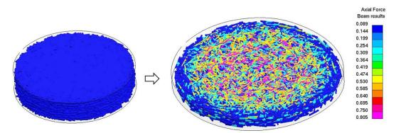
Figure 6: Deformation behaviour and axial forces in beam elements
