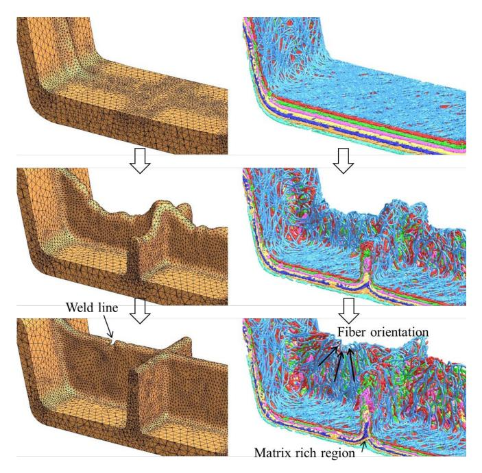
Figure 11: EFG r-adaptive mesh refinement and beam orientation behaviour
