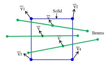
Figure 3: Constraint of multiple beam elements in one solid element
