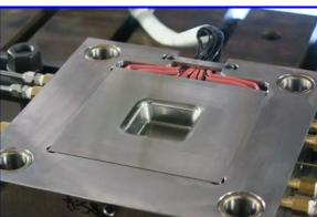
Figure 13: Punch and die shapes used in experiment
