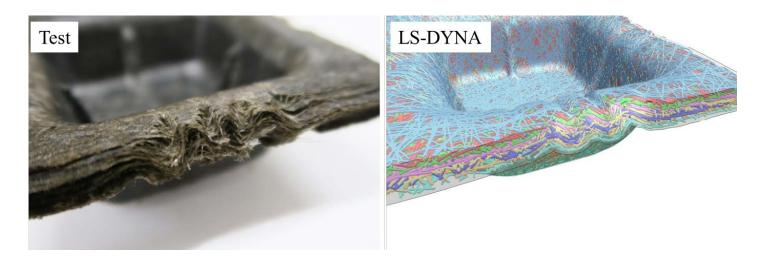
Figure 14: Charge wrinkling mid-way through the punching process
