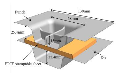
Figure 9: Compression molding model to form cross-rib shaped component
