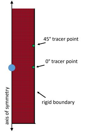
Figure 9: 2-D axisymmetric mesh showing the location where impulses were recorded.
