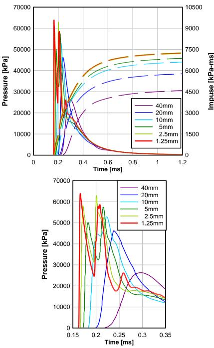
Figure 4: Pressure and impulse histories at a point opposite the charge on a reflecting wall (2-D axisymmetric).
