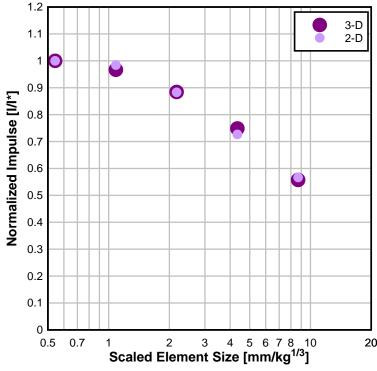
Figure 12: Comparison of mesh convergence for 2-D and 3-D simulations.
