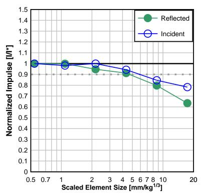
Figure 7: Normalized incident and reflected impulses taken at the same standoff.
