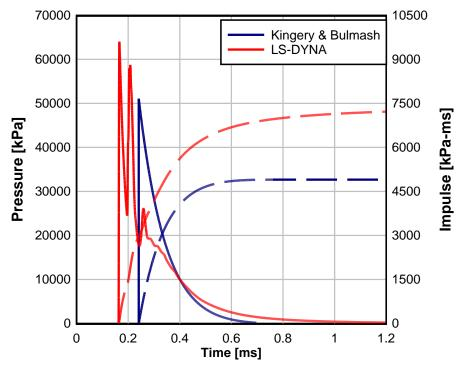
Figure 3: Comparison of waveforms from Kingrey & Bulmash with high fidelity LS-DYNA result.
