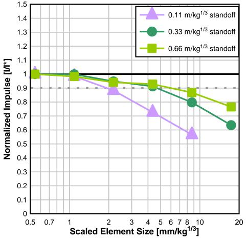
Figure 8: Normalized reflected impulse taken at different standoff distances from the charge.
