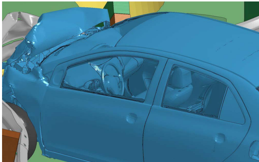
Figure 5. SIDE VIEW OF VEHICLE AFTER COLLISION WITH 15° IMPACT ANGLE.
