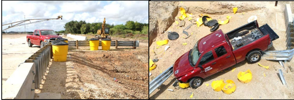
Figure 13. MASH Test 3-33 (sloped terrain) at impact and final vehicle position.
