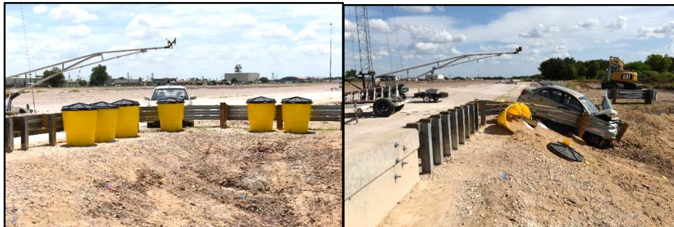
Figure 12. MASH Test 3-32 (sloped terrain) at impact and final vehicle position.
