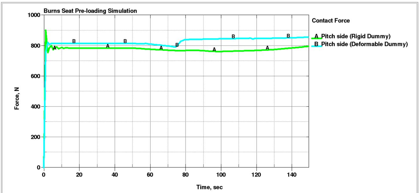
Fig 7. Contact force between the dummy and seat on the pitch side
