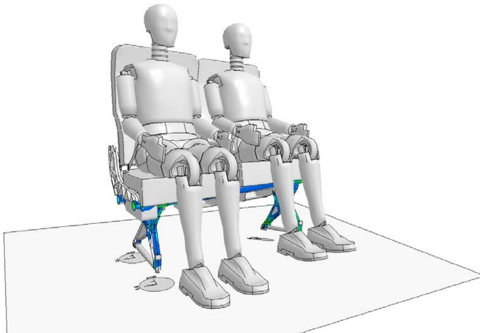
Fig 1. Dummies on pre-loaded aircraft seat
