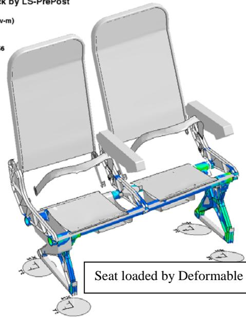
Seat loaded by Deformable Dummy
