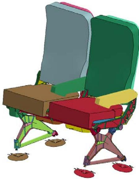
Fig 5. Seat Only subjected to pre-loading as integrity test
