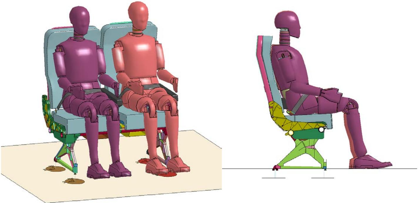
Fig 3. Dummies positioned on Burns aircraft seat
