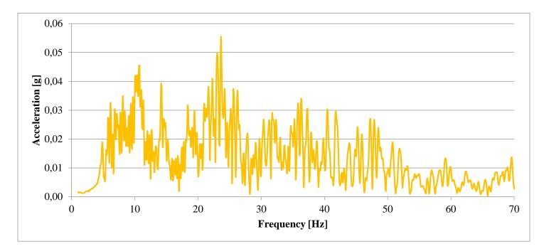
Figure 11: Input Profile – Shock Test
