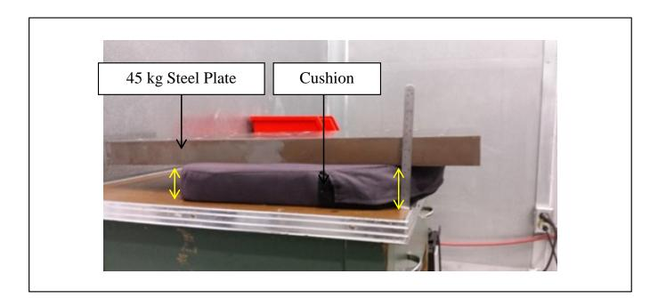
Figure 5: Compression Test Setup
