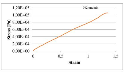
Figure 3: HS-70 Ethafoam Stress-Strain Curve
