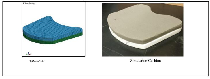
Figure 4: Simulation Model of the Cushion
