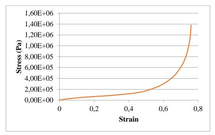
Figure 2: T41 Temperfoam Stress-Strain Curve
