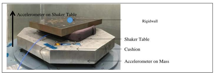
Figure 7: Shaker Table Setup
