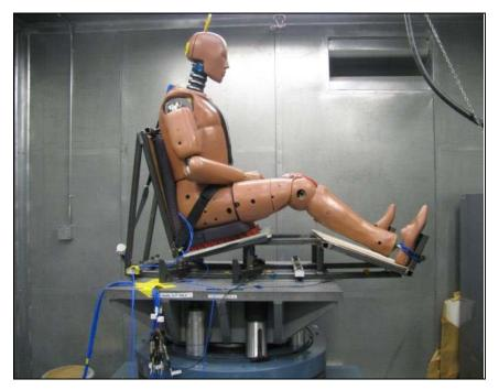
Figure 12: Shock Test with Dummy
