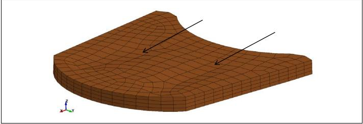
Figure 10: Localized Compression on the T41 Temperfoam Cushion
