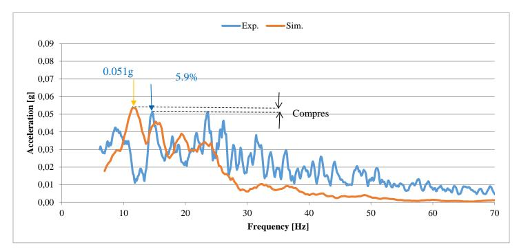
Figure 13: Shock Test Simulation Results on the Pelvis
