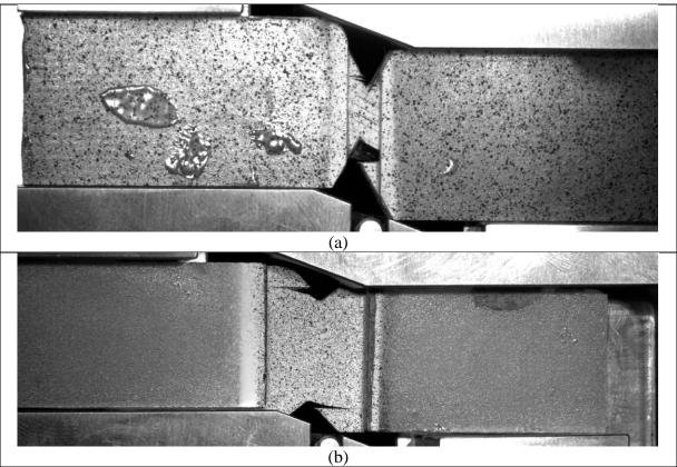
Figure 5. Failed Iosipescu shear test specimens (a) 1-2 plane and (b) 1-3 plane
