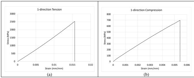
Figure 3. 1-direction model curves (a) tension response and (b) compression response
