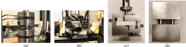
Figure 1. (a) Hydraulic grips for tension tests, (b) DIC equipment, (c) Iosipescu shear test fixture, and (d) Combined loading compression fixture
