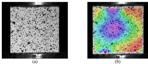
Figure 2. 3-direction compression test (a) Speckled specimen and (b) Resulting longitudinal strain field.
