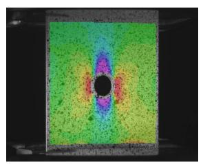
Figure 9. Open-hole tension longitudinal strain field
