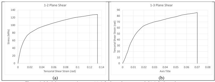
Figure 4. Model stress-strain curve (a) 1-2 plane shear test and (b) 1-3 plane shear test
