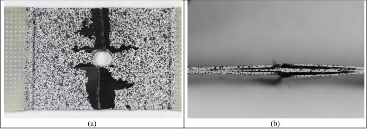
Figure 8. Failed open-hole tension experimental specimen (a) front view and (b) side view
