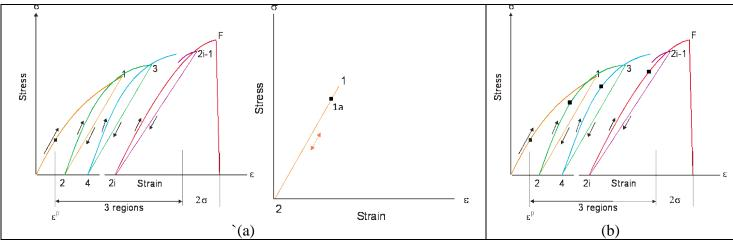
Figure 6. Damage characterization testing procedure (a) Coupled damage procedure and (b) Uncoupled damage procedure
