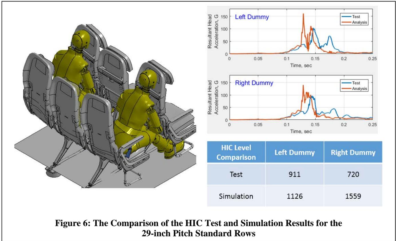
**Figure 6: The Comparison of the HIC Test and Simulation Results for the 29-inch Pitch Standard Rows**
