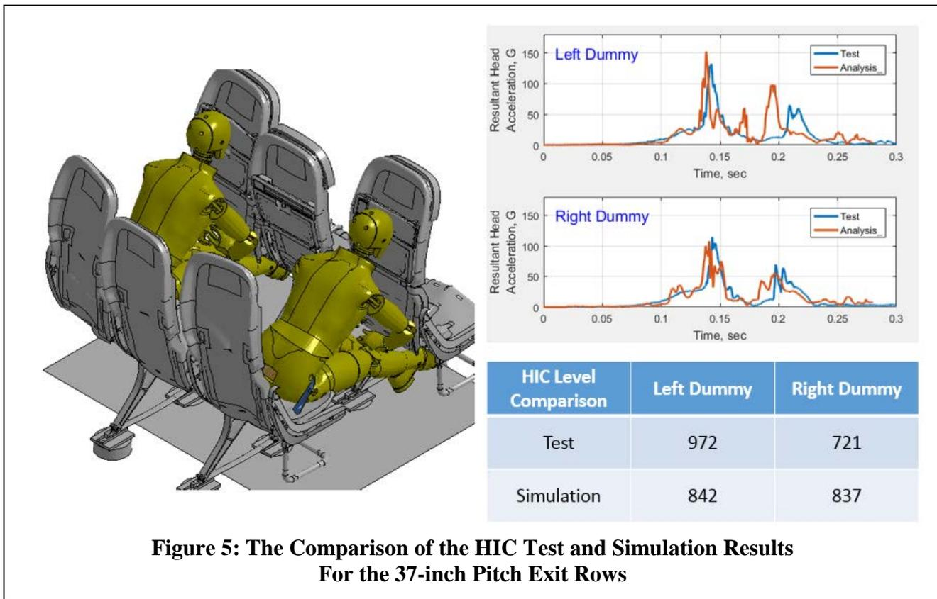
**Figure 5: The Comparison of the HIC Test and Simulation Results For the 37-inch Pitch Exit Rows**
