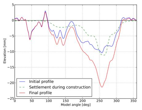
Figure 3: Analysis A – circumferential foundation profiles
