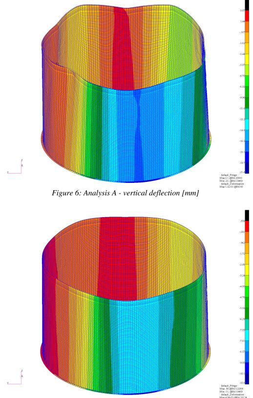
Figure 7: Analysis B - vertical deflection [mm]
