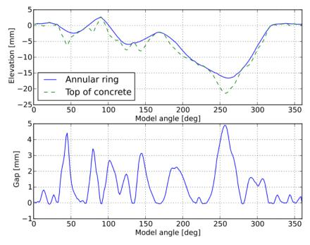
*Figure 8: Analysis A – contact between the annular ring (bottom of strake 1) and the top surface of the concrete foundation*
