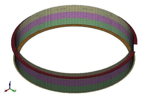
*Figure 2: Construction up to third strake and temporary wind girder installation*
