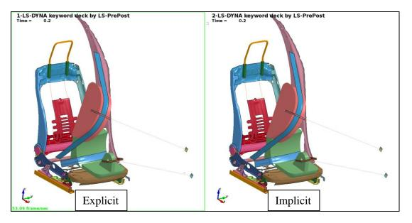
Figure 4 Final deformed state of seat structure
