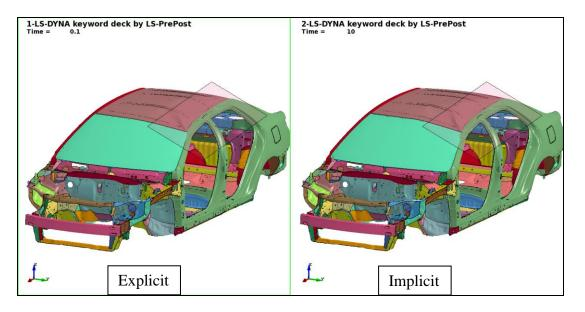
Figure 3 Final deformed state comparison
