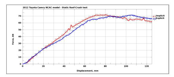
Figure 2: Force-Displacement plot
