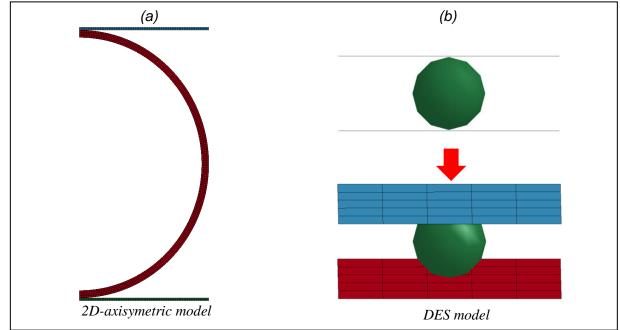
Figure 5: Compression test 2D-axisymetric model (a) and DES model (b)
