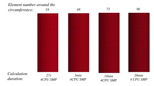
Figure 4: Mesh and performance studies with the vibratory explicit method
