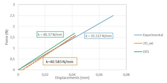
*Figure 6: Force-displacement curve of the experimental (blue), hollow 2D-axisymetric (red) and full DE (green) spheres for small strains*
