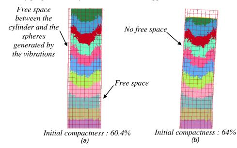
Figure 9: Comparison of the spheres behavior in the vibrating cylinder for unconstrained spheres (a) and constrained ones (b)
