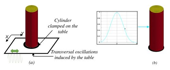
Figure 3: Load illustration for numerical mode detection: (a) transversal vibration, (b) pulse
