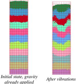
Figure 7: Gravity compaction illustration
