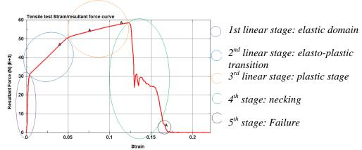
Figure 15: Description of the various stages of the compact stacked DES elasto-plastic behavior
