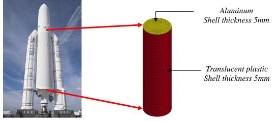
Figure 2 : Cryogenic tank simplified model
