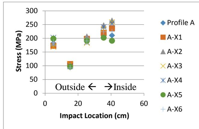
Figure 7: Max stress as a function of impact location for purely elastic models of Profile A and modified profiles.
