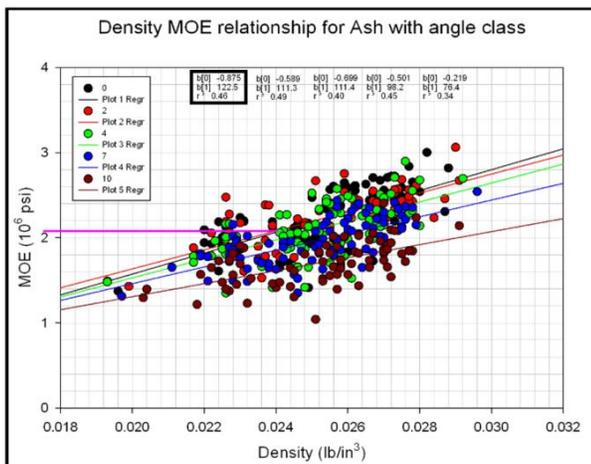
Figure 2: MOE variance with density for ash wood dowel testing
