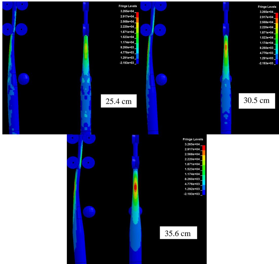
Figure 9: The 4° constant taper slope models showing stress contours. The dimension in the figure is the taper starting position as measured from the base of the knob.
