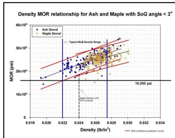
Figure 3: MOR variance with density for ash and maple wood dowel testing
