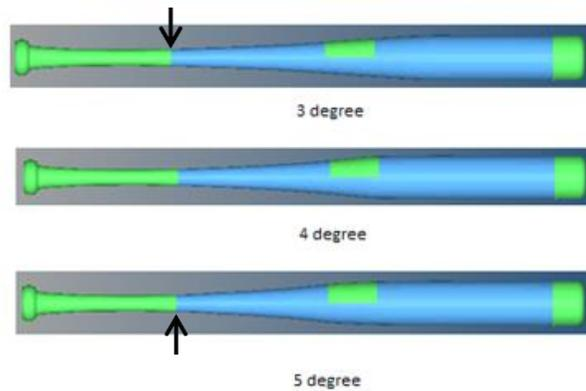
Figure 8: Finite element models of bats with 3°, 4°, and 5° constant taper slopes and taper starting at 25.4 cm (10 in.) as measured from the base of the knob
