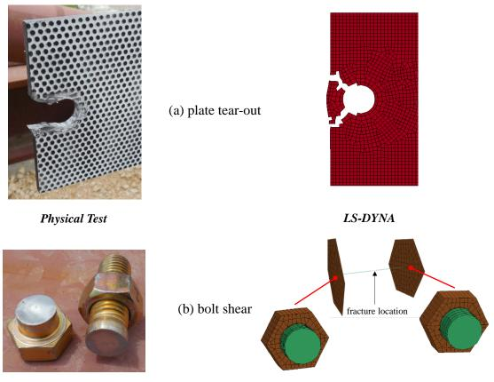
Fig. 14: Comparison of failure modes in the simplified bolted connection specimens modelled with LS-DYNA and the physical tests, (a) plate tear-out, (b) bolt shear
