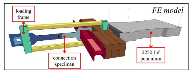
Fig. 12: Finite element model used to replicate the pendulum tests
