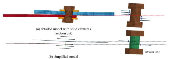
Fig. 8: Bearing forces, (a) detailed model with solid elements, (b) simplified model
