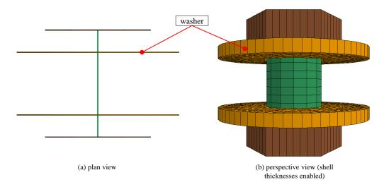
Fig. 5: Finite element model of the bolt/nut including washers, (a) plan view, (b) perspective view
