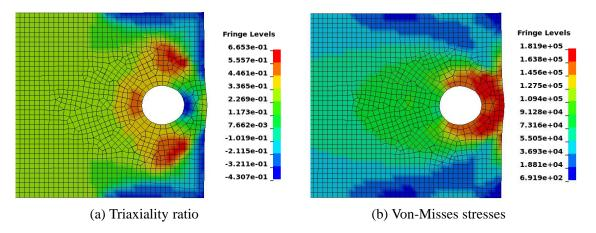
Fig. 10: Triaxiality ratio and von-Mises contours on a plate that is bearing against a bolt (bolt not shown for clarity)
