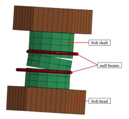
Fig. 9: Interaction of the bolt-shaft with the null beams in the simplified connection models
