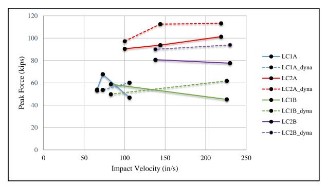
Fig. 13: Peak force versus impact velocity, experimental data and LS-DYNA simplified simulations
