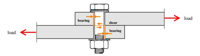
Fig. 1: Bolted connection loaded in direct shear
