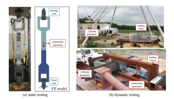
Fig. 3: Testing apparatus used for the connection tests; (a) static testing, (b) dynamic testing
