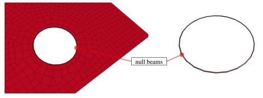
Fig. 7: A view of the plate depicting the null beam elements placed around the bolt-hole
