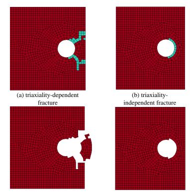
*Fig. 11: Plate tear-out fracture, (a) triaxiality-dependent fracture, (b) triaxiality-independent fracture*
