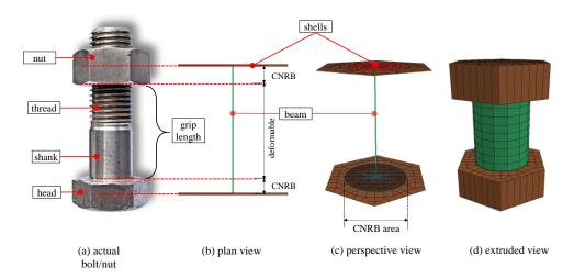
*Fig. 4: Finite element model of bolt/nut, (a) actual bolt/nut, (b) plan view, (c) perspective view, (d) extruded view*
