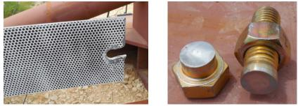
(a) plate tear-out failure
