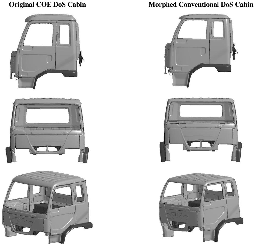
**Figure 1. Original COE DoS cabin versus morphed conventional cabin models.**
