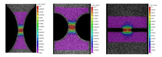
Fig. 6: DIC data from tensile testing of flat-notched-specimens.
