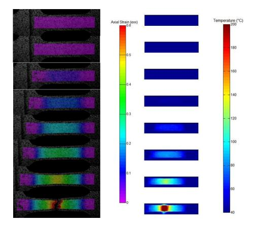
Fig. 8: DIC processed images recorded by the visual camera and IR camera images at different times during the test.
