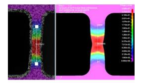
Fig. 5: DIC data and numerical simulation of a tensile test.
