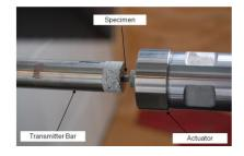
Fig. 3: Intermediate strain rate apparatus.
