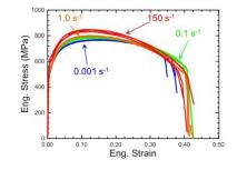
Fig. 4: Tensile stress strain curves for HHS at different strain rates.
