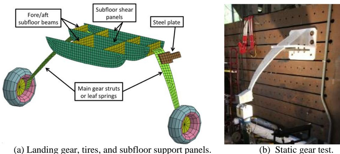
(a) Landing gear, tires, and subfloor support panels.
