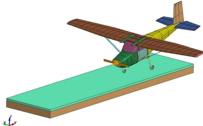
Figure 2. LS-DYNA model representing the Test 2 configuration.
