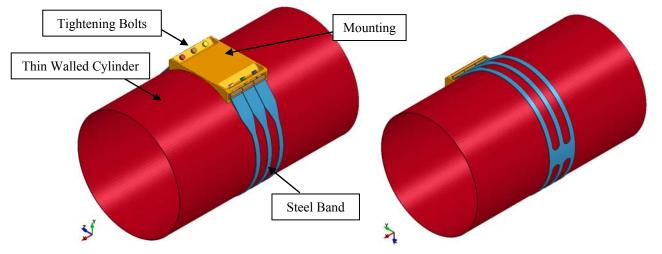
Figure 1: Band clamp assembly model
