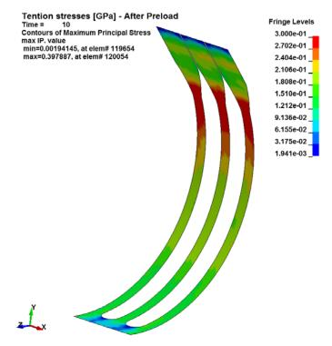
Figure 7: Stress distribution along the band after preload for  $\mu$ =1
