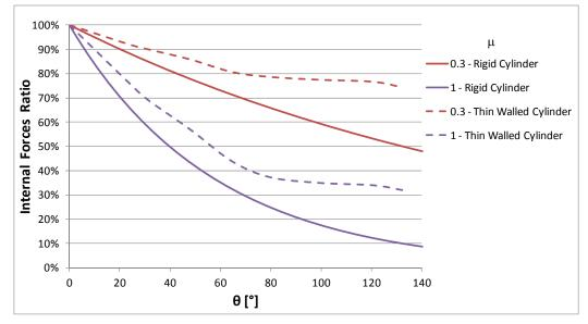
Figure 9: A comparison between a rigid cylinder and a thin walled elastic cylinder
