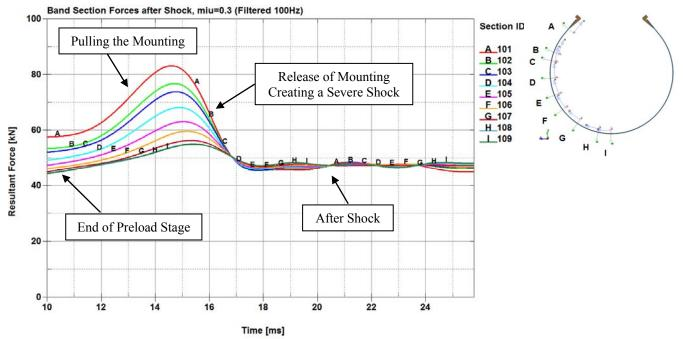
Figure 12: Internal tension forces in the band subjected to severe shock with  $\mu$ =0.3
