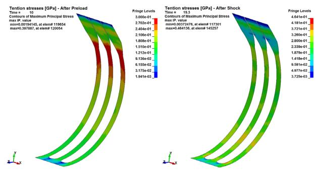
Figure 11: Stress distribution in the band for  $\mu=1$  after preload stage (left) and after the shock (right)
