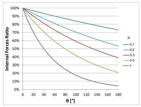
Figure 3: Theoretical force decrease along the band for various coefficients of friction
