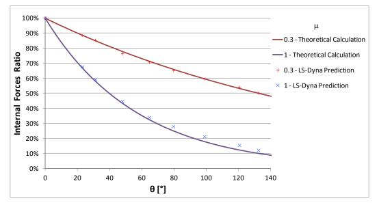
Figure 10: A comparison between theoretical calculation and LS-DYNA Prediction for a rigid cylinder
