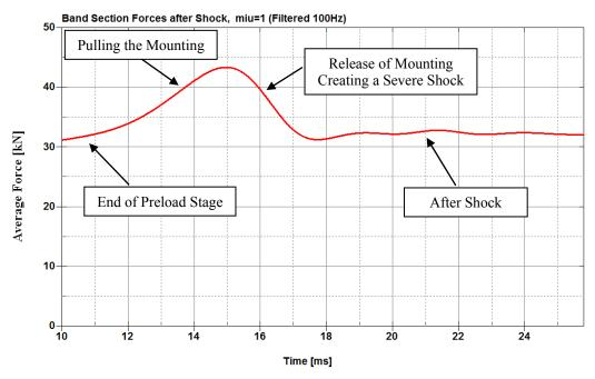
Figure 15: Average of the internal tension forces in the band for  $\mu$ =1
