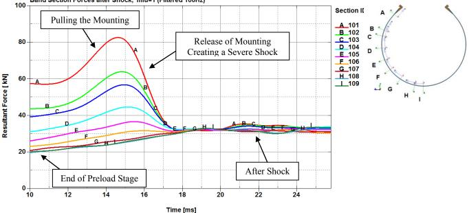
Band Section Forces after Shock, miu=1 (Filtered 100Hz)
