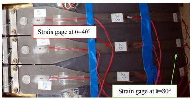
Figure 4: Strain gages attached to the band
