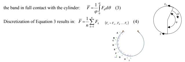
Calculating an average force (Equation 4), shows that the final uniform internal force is equal to the average of the distributed internal forces in the band at the end of the preload stage. This result can be demonstrated in **Figure 15** for  $\mu$ =1.
