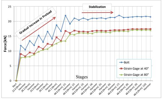
Figure 5: Experimental measurements for assembly process using stages of hammering
