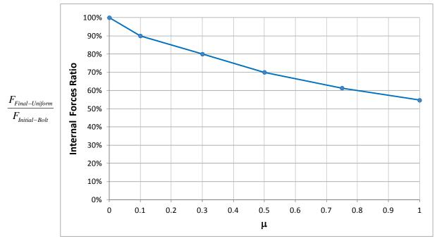
Figure 14: Maximal decrease of the initial preload force under dynamic loading conditions
