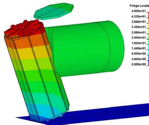
**Figure 7:** Velocity field [m/s] on overpack and impactor 80 ms after impact start
