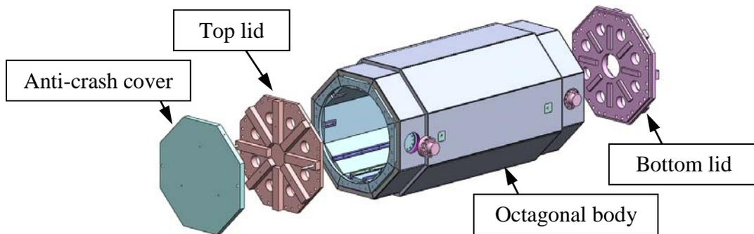
**Figure 2:** General view of the TN NOVA™ overpack
