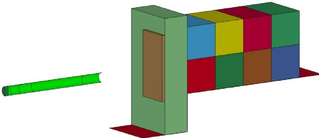
**Figure 9:** Finite element model of the missile calibration test
