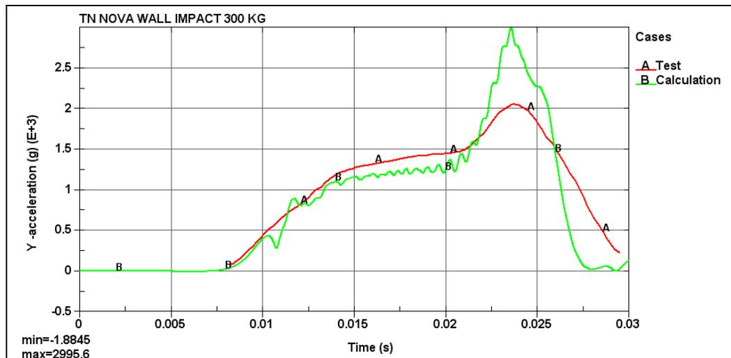
**Figure 10:** Simulated/real missile calibration test – Missile acceleration vs. time
