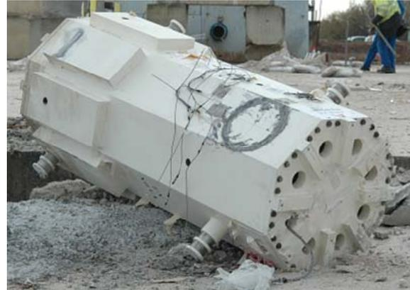
**Figure 15:** Simulation/real test - State of overpack after missile impact
