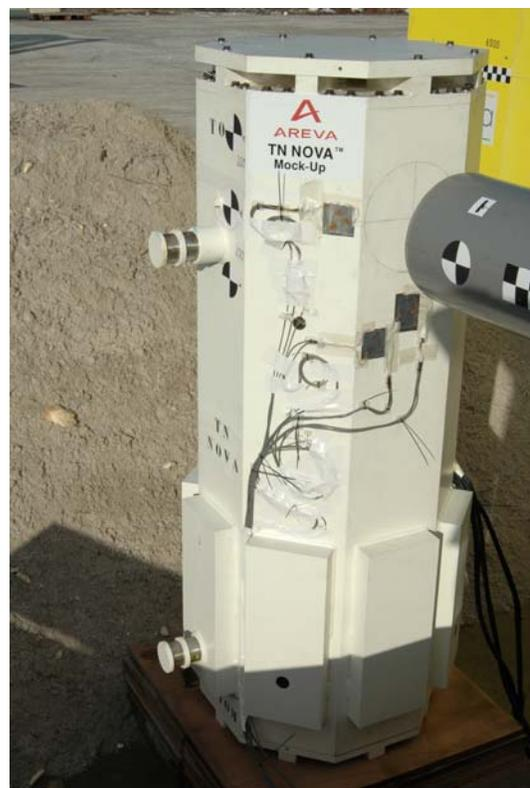
**Figure 11:** Real test – TN NOVA™ mock-up before missile impact
