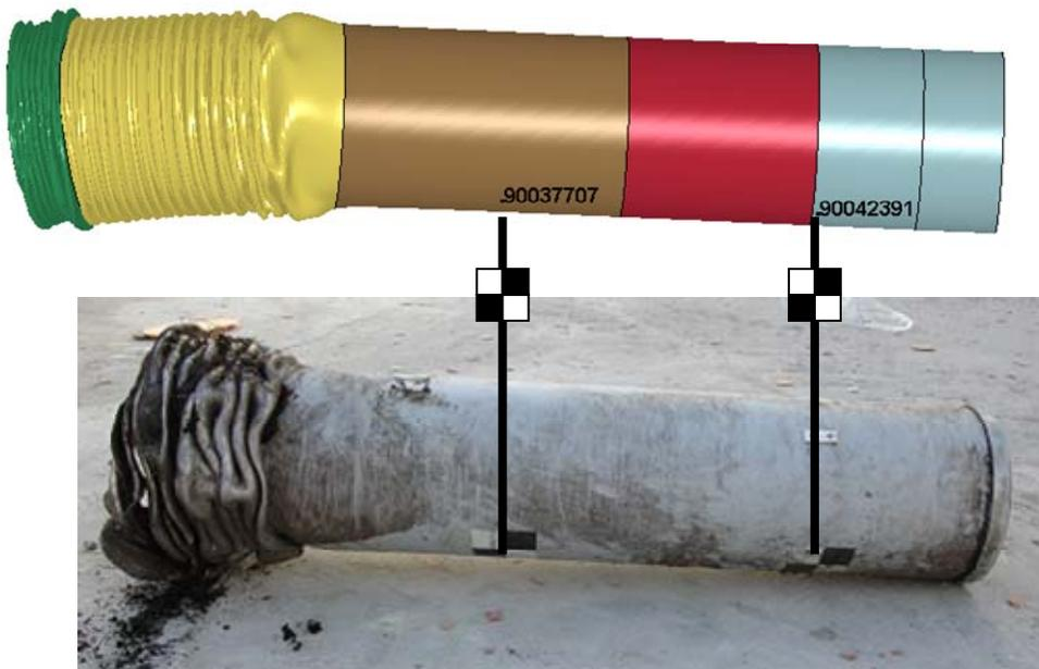
**Figure 14:** Simulation/real test – Deformed missile after impact
