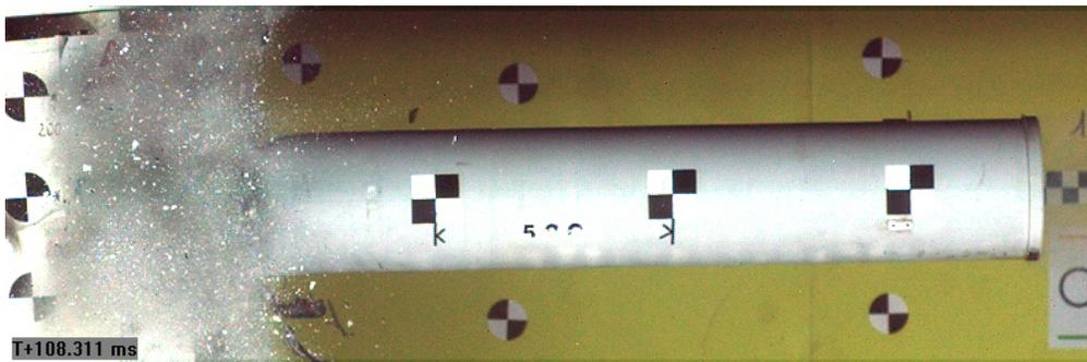
**Figure 13:** Real test – Missile impacting TN NOVA™ mock-up
