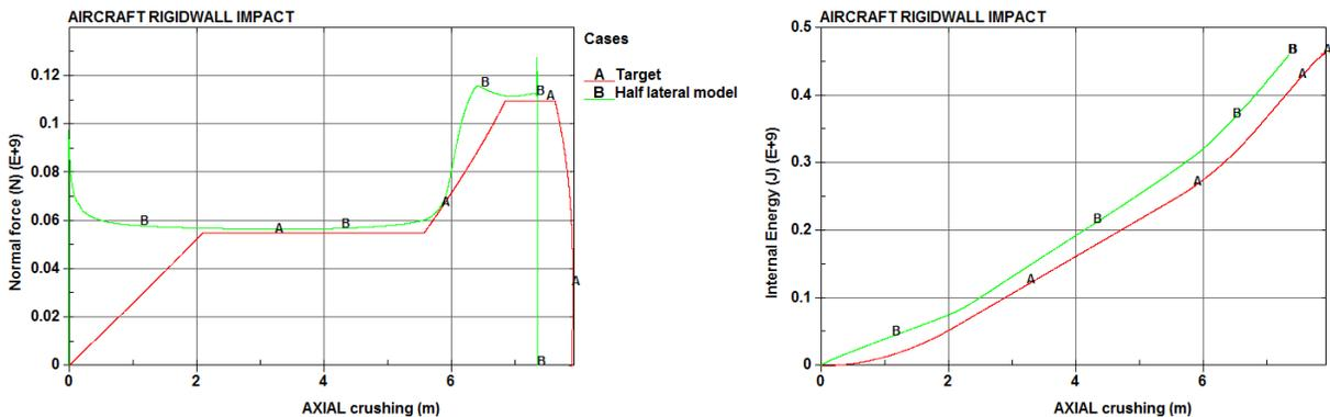
**Figure 5:** Impactor compared to specified aircraft in terms of load and internal energy vs. axial crushing
