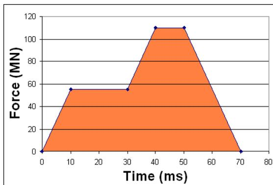
Figure 3: Aircraft crash – Specified impact force vs. time curve
