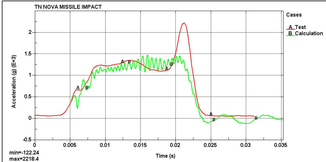
**Figure 12:** Simulated/real final test on the TN NOVA™ mock-up – Missile acceleration vs. time
