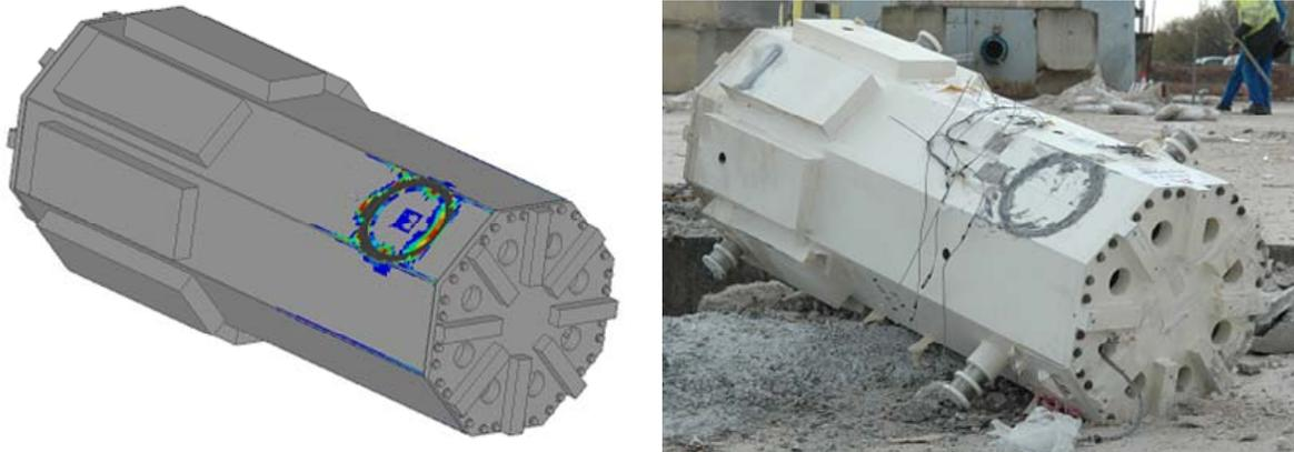
**Figure 15:** Simulation/real test - State of overpack after missile impact
