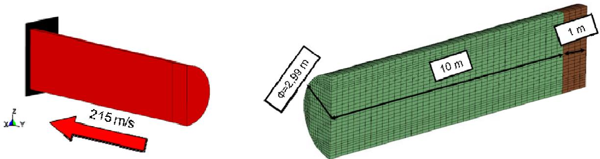
**Figure 4:** Finite element model of the impactor
