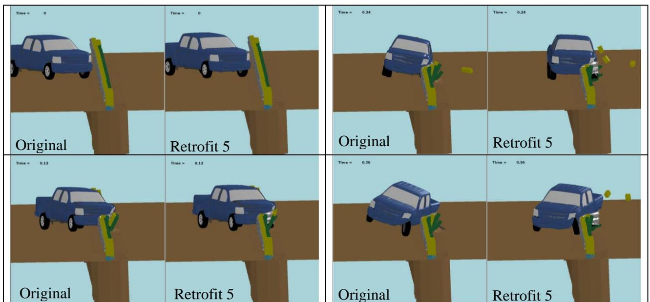
Figure 3 - Simulation Comparisons of the Original Design & Half Blockout Thrie-Beam Option
