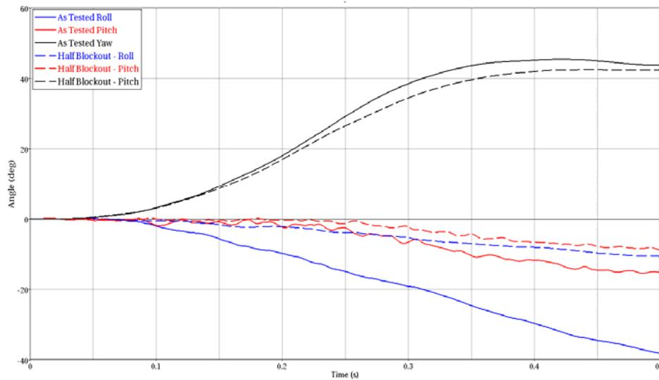
Figure 2 – Roll, Pitch, & Roll Comparisons of Original Design & Half Blockout Thrie-Beam Option
