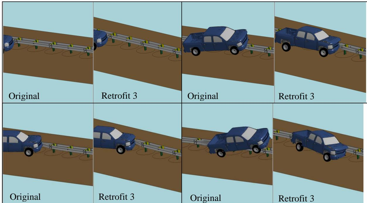
**Figure 4 - Simulation Comparisons of the Original Design & the Three Inch Increased Height.**
