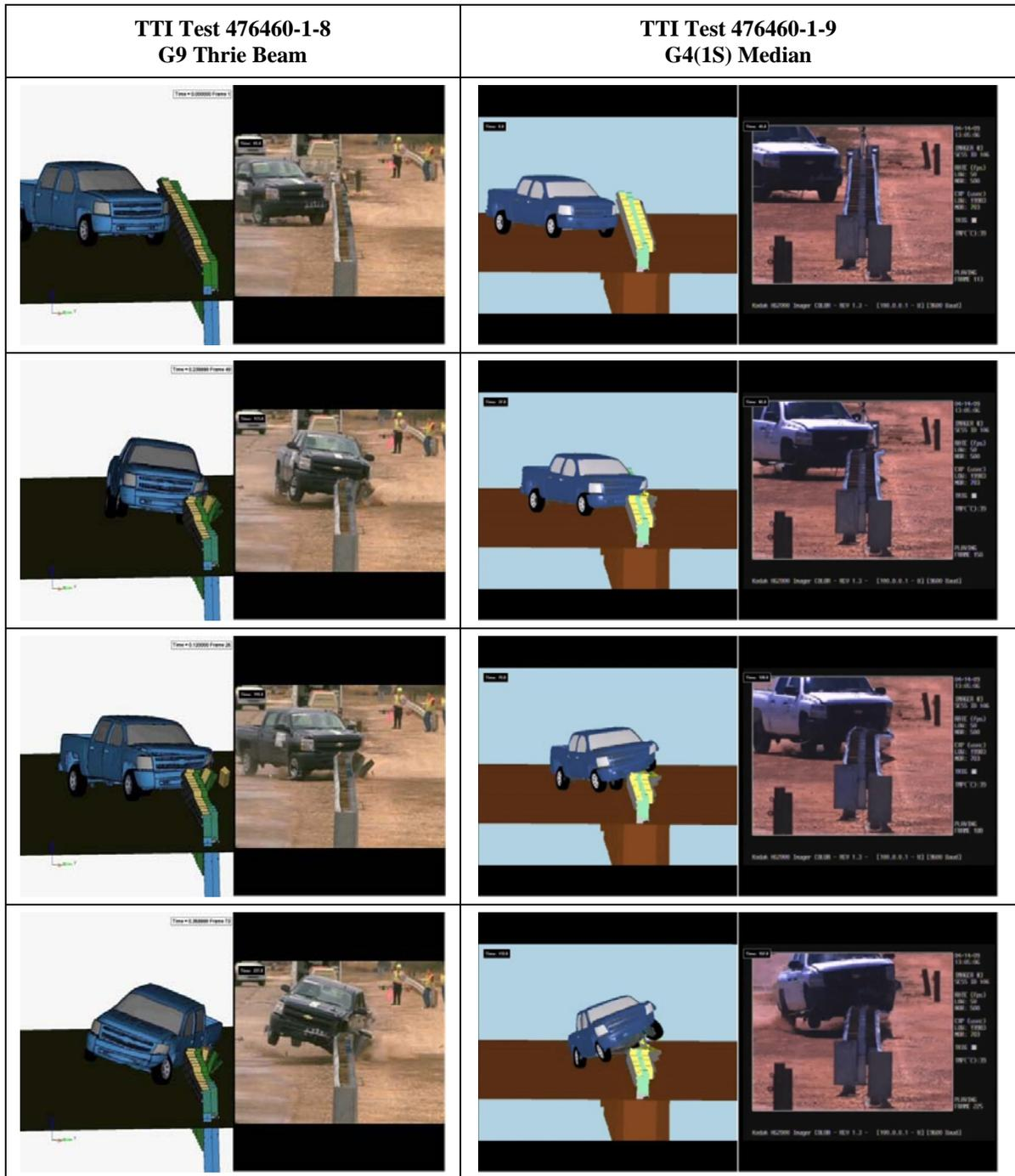
Figure 1 – Side by Side Comparisons of Test and Simulation for the two Barriers Analyzed
