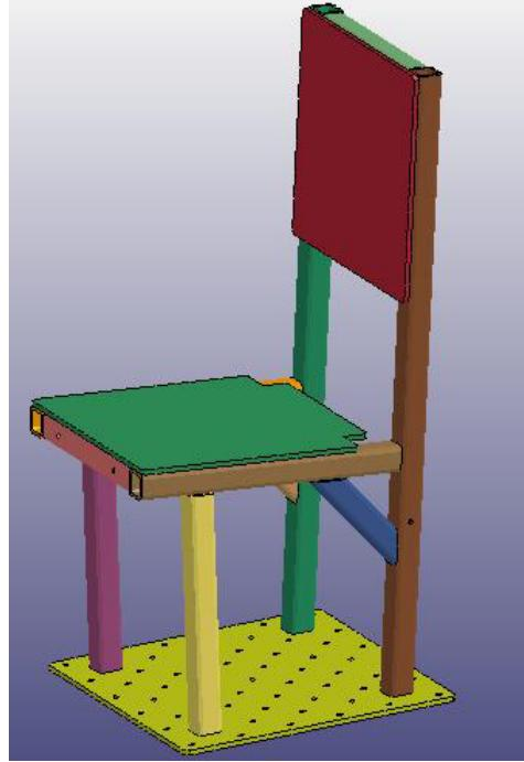
**Figure 7:** Rigid seat finite element model
