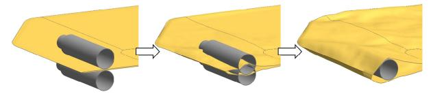
Figure 10: Double inflator models insert method.
