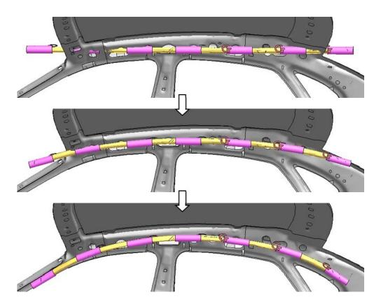
Figure 11: Fitting curtain airbag to roof side rail
