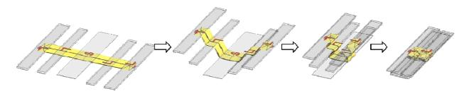
Figure 7: Z-folding performed by load type tools.
