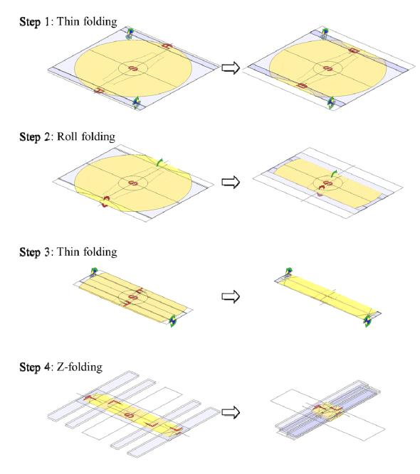
Figure 6: Driver airbag folding.
