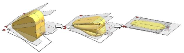
Figure 8: Passenger airbag folding simulation
