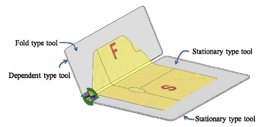
Figure 2: Four tools make up the thin-folding model.
