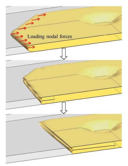
Figure 4: Tuck folding performed by nodal forces
