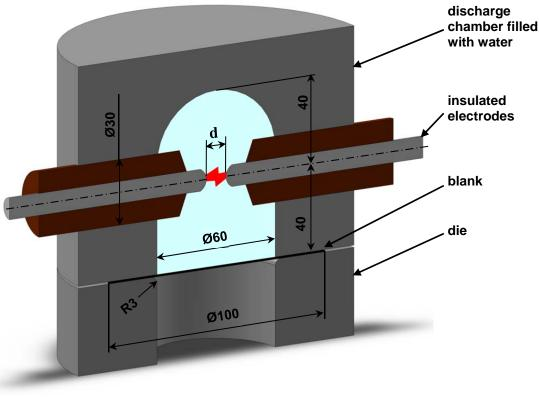
Figure 4. Tool for EHF process
