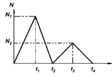
Figure 5. Energy deposition law:  $t_1 = 24 \ \mu s$ ,  $t_2 = 49 \ \mu s$ ,  $t_3 = 76 \ \mu s$ ,  $t_4 = 102 \ \mu s$ ,  $N_1 = 9.1 \ MW$ ,  $N_2 = 4.9^{\circ}MW$
