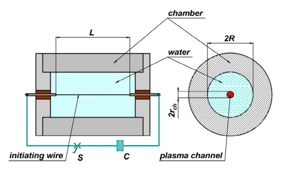
Figure 1. The scheme of the test equipment
