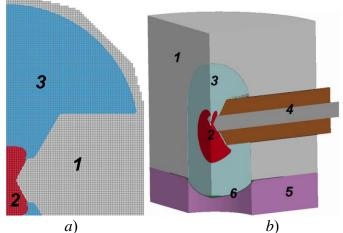
Figure 6. ALE mesh and deformation of the fluid parts and the blank at the moment 245 μs (a: 1 – vacuum mesh, 2 – plasma MM group, 3 – water MM group; b: 1 – discharge chamber, 2 – plasma bubble, 3 – water, 4 – electrode, 5 – die, 6 – deforming blank)
