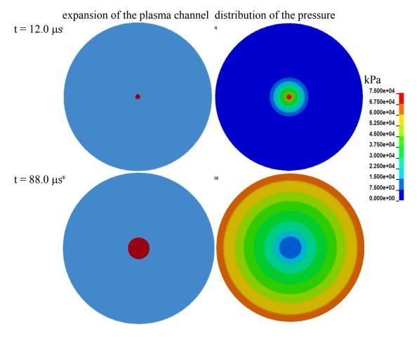
Figure 2. Simulation results for cylindrical chamber
