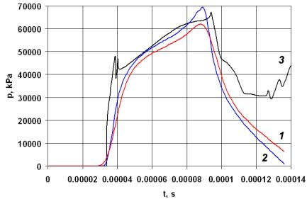
Figure 3. Pressure on the cylindrical wall of the chamber: 1 – LS-DYNA, 2 – numerical results from one-dimensional finite-difference problem, 3 – experimental results
