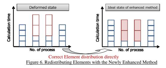
Applying this enhanced domain decomposition on the aforementioned ODB model; the distribution of elements to each subdomain has been readjusted as expected. Figure 7 shows those subdomains in Zone B with larger deformed element have less total number of element per domain; each subdomain in Zones A and C with less deformed element has more total number of element allocated.
