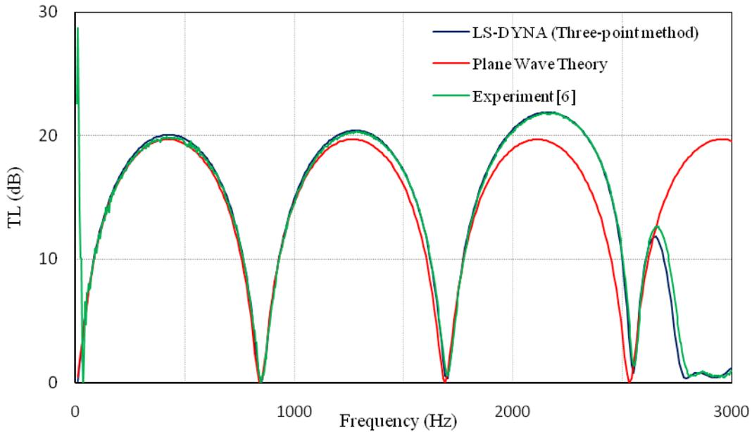
Figure 4. Transmission Loss Comparisons (Three point method)
