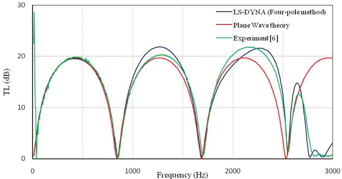
Figure 5. Transmission Loss Comparisons (Four pole method)
