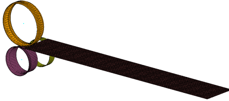
Figure 6. Meshed strip before entering the first forming station. Note the mass element at the center of each roll.
