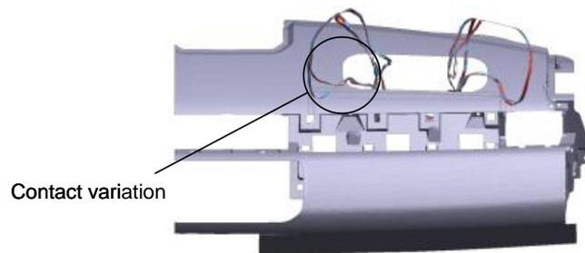
Figure 8. Variable contact of airbag strap at 23ms
