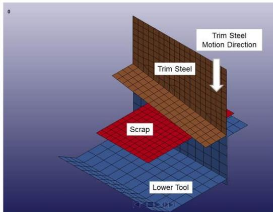
Figure 1-1 Simulation model
