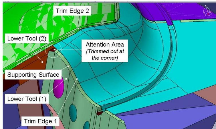
Figure 2-2. Details of the tools/panel near a corner of two trim edges
