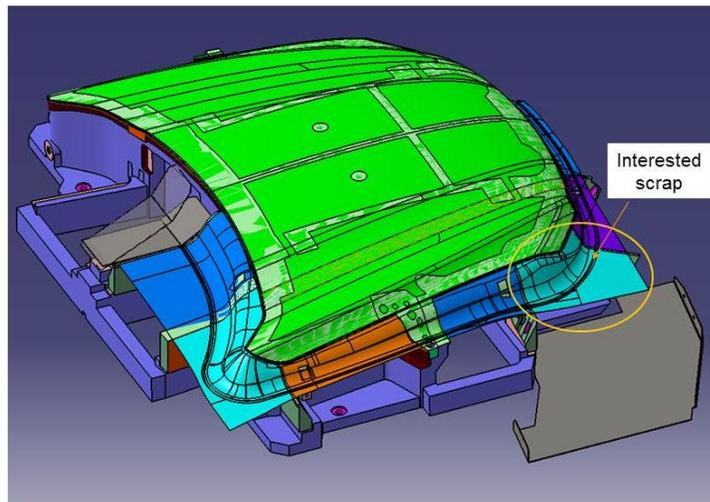
Figure 2-1. Overview of a die design for a hood outer panel
