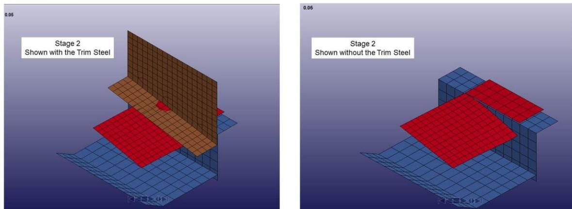
Figure 1-4. Final stage of the trimming (right – trim steel not shown)
