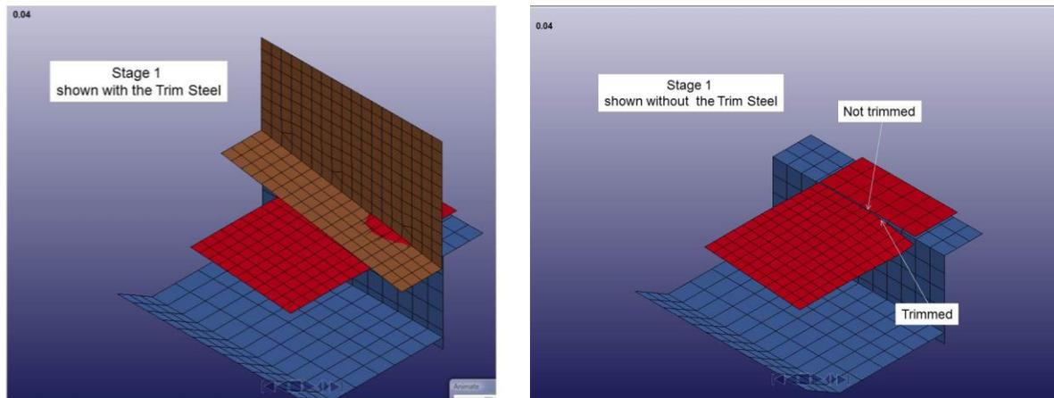
Figure 1-3. Early stage of trimming (right - trim steel not shown)
