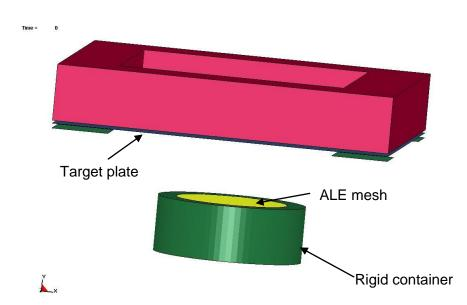
Sand is modeled as LS-DYNA Discrete Elements. TNT charge is using \*MAT\_HE + \*EOS\_JWL and ALE element formulation 11. The other fluid is air using \*MAT\_NULL+\*EOS\_LINEAR\_POLYNOMIAL. The coupling between sand and TNT charge uses \*ALE\_COUPLING\_NODAL\_CONSTRAINT card with both velocity and acceleration constrained. The resultant deflection on the plate agrees well with CONWEP results obtained through \*LOAD\_BLAST cards.
