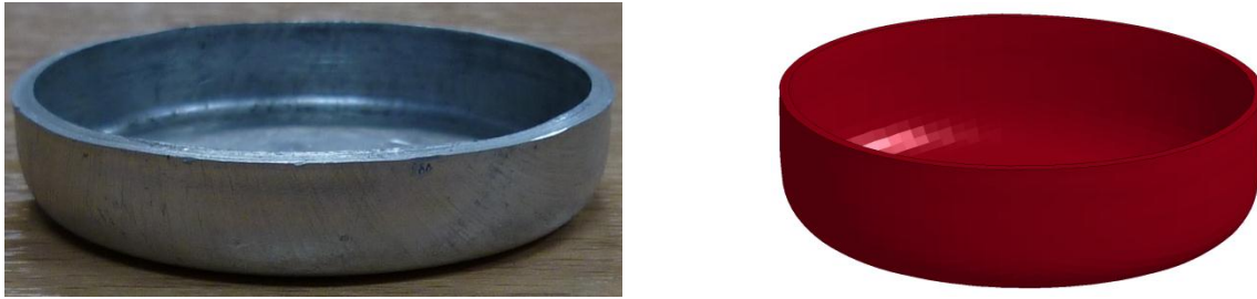
Fig.5. Exterior view of the detail: Left: experiment, right: LS-DYNA simulation
