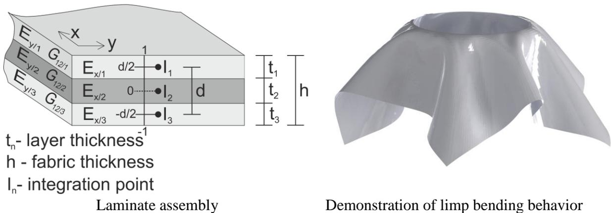
Figure 4 Laminate assembly and limp bending behavior
