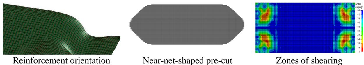
Figure 8 Near-net-shaped pre-cut and zones of shearing
