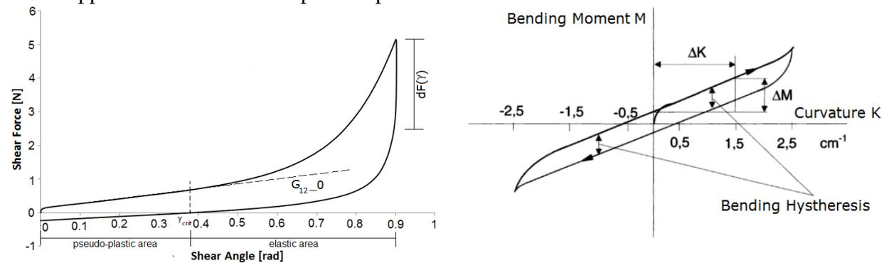
Shear force vs. shear angle hysteresis
