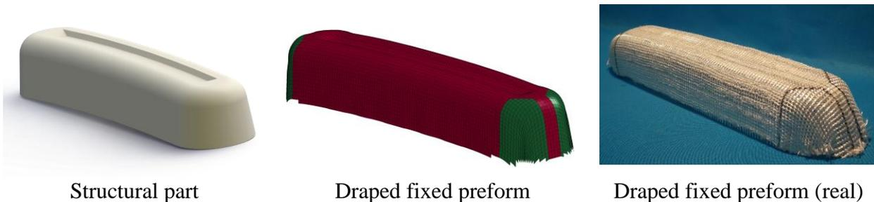
Figure 11 Comparison of structural part and drape simulation
