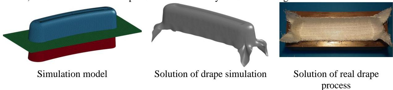
Figure 7 Solution of first drape simulation
