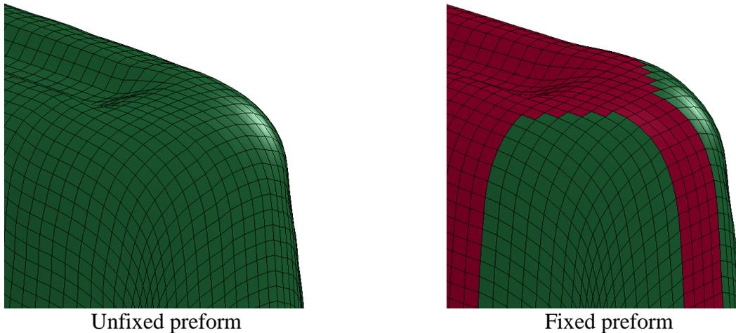
Figure 10 Comparison of reinforcement orientation (unfixed and fixed preform – gravitational load)
