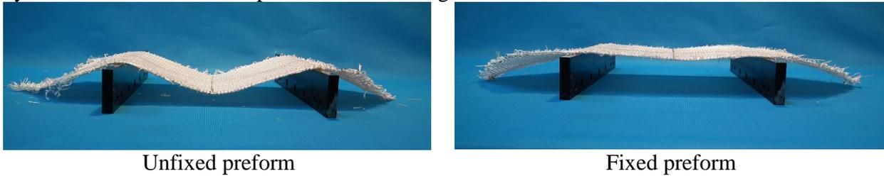
Figure 9 Comparison of preform stability (unfixed and fixed preform)
