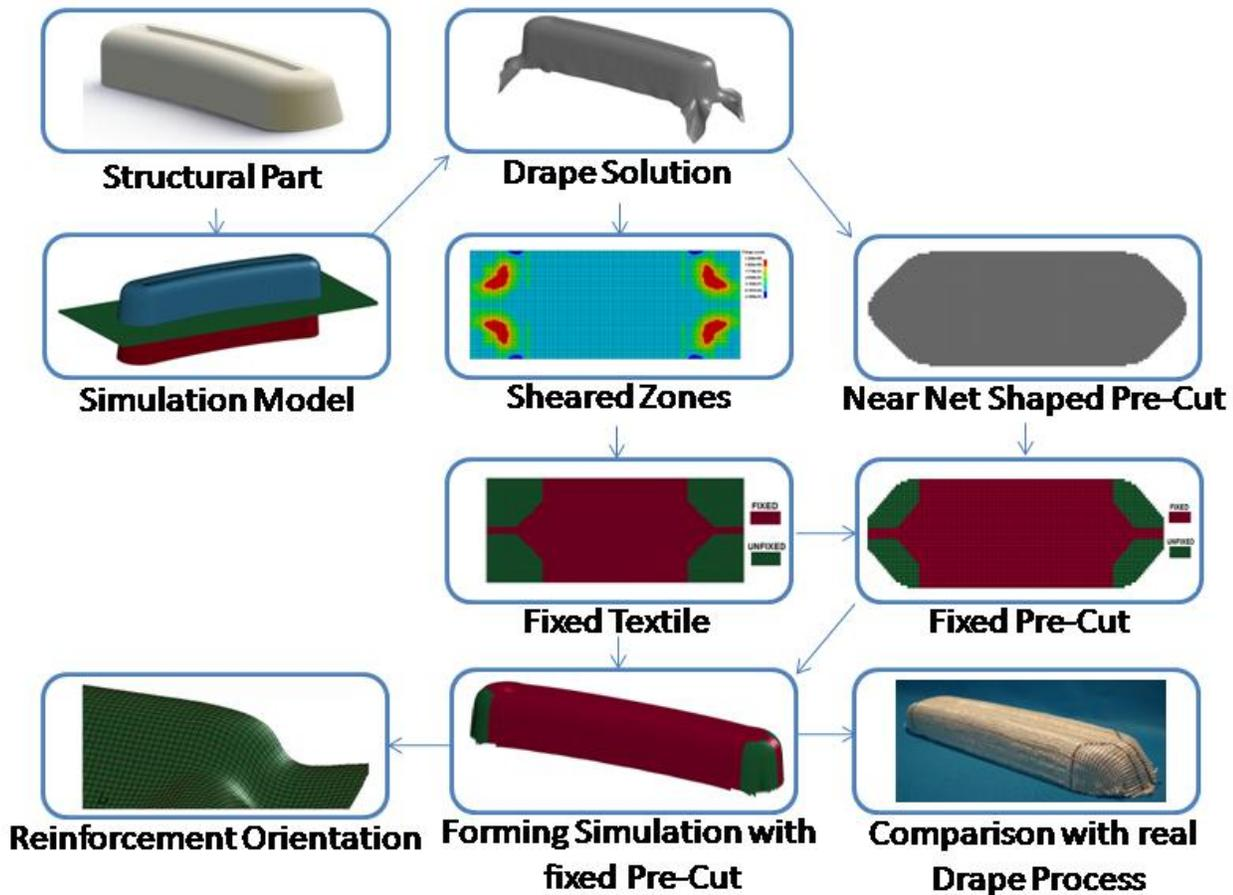
Figure 5 Process chain for preform development
