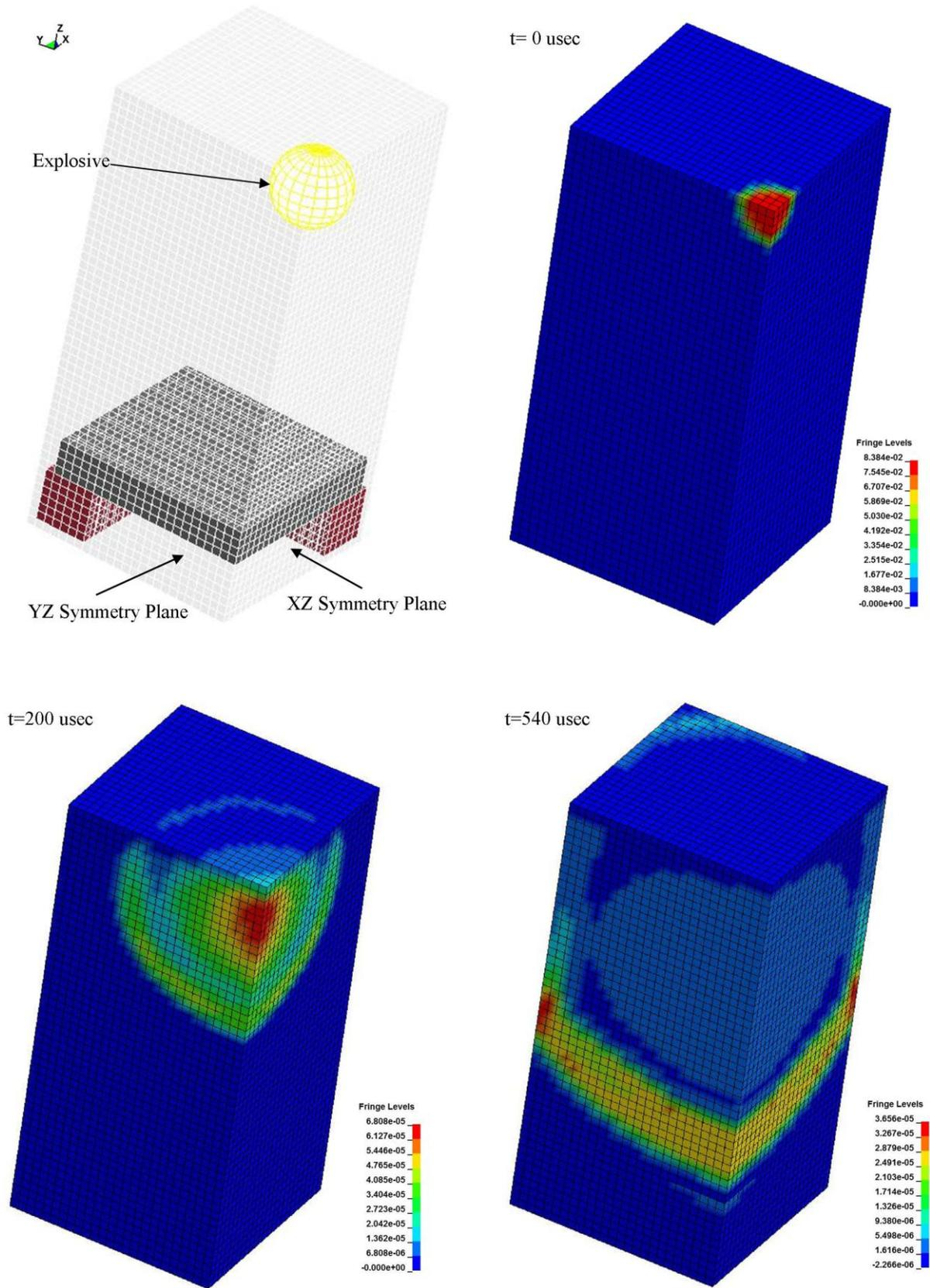
Figure 2. Time sequence of pressure fringes showing wave propagating from the explosive source
