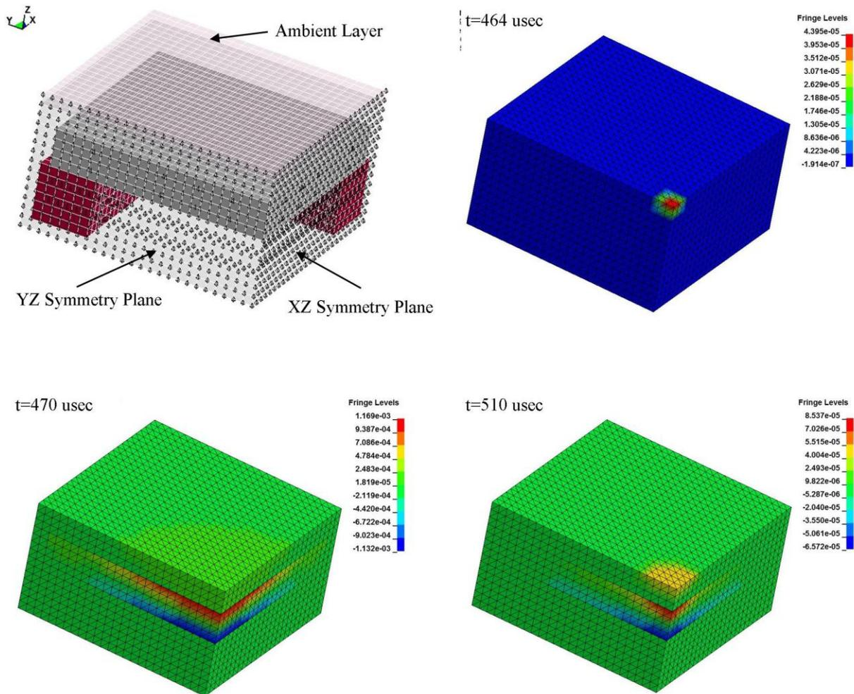
Figure 3. Time sequence of pressure fringes showing wave propagating from the ambient layer
