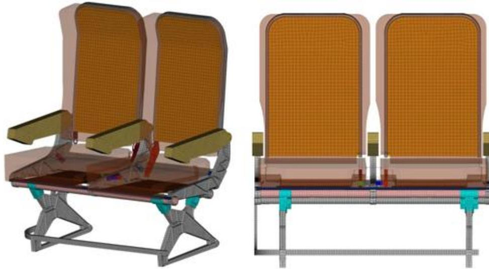
Figure 6 FE Model of Typical Aircraft Seat
