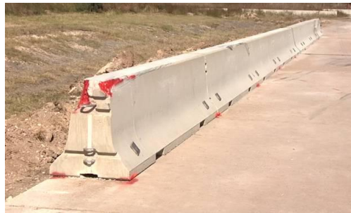
Figure 6 Pinned-down F-shaped temporary barrier before testing.
