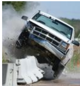
(b) Lifting of barriers observed in modified simulation and test
