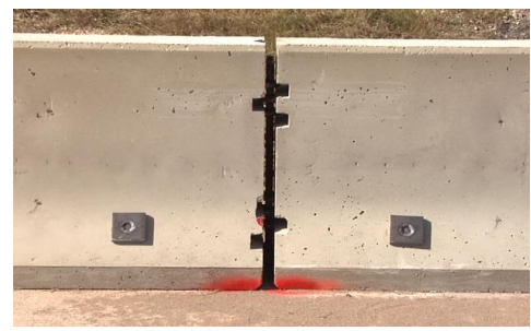
Figure 6 Pinned-down F-shaped temporary barrier before testing.
