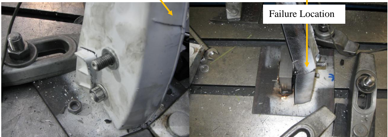
Figure 19 Crack Initiation from Test & FEA
