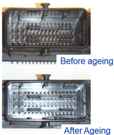
Fig.3: Header walls deformation before and after thermal ageing
