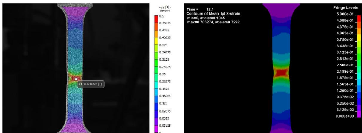
Fig.9: Comparison of strain fields from DIC experiment and simulation for uniaxial tension.
