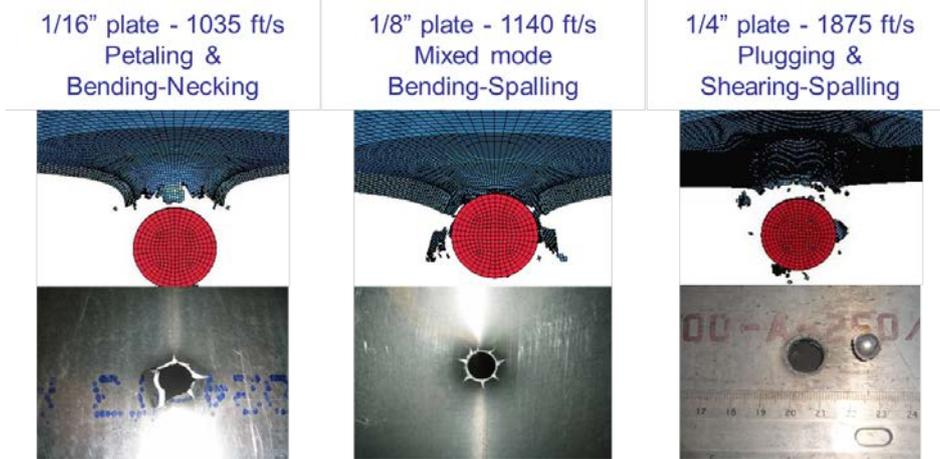
Fig. 1: Failure mode transition from petaling to plugging with target thickness and projectile energy.
