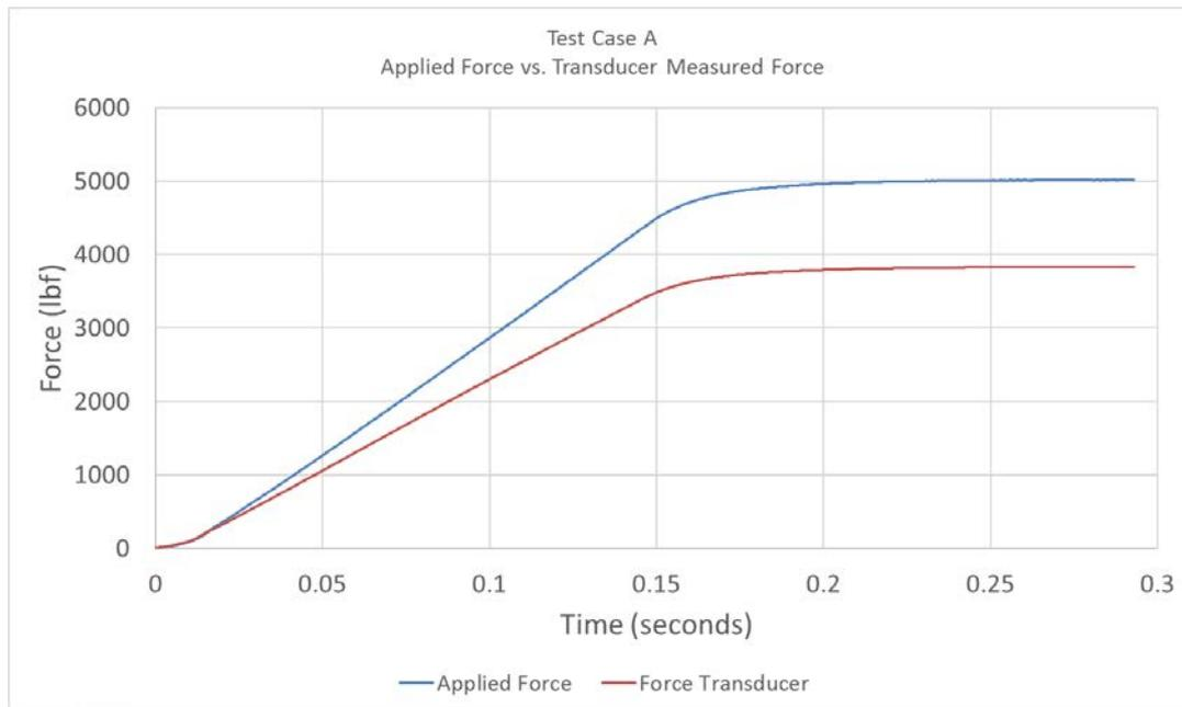
Fig.4: Graph of the applied force to the entire bolted joint and the load measured in the force transducer for Test Case A.
