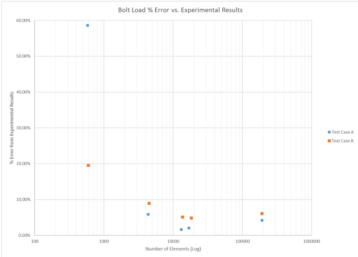
Fig.9: Percent difference in bolt load between experimental and finite element data for various mesh densities.
