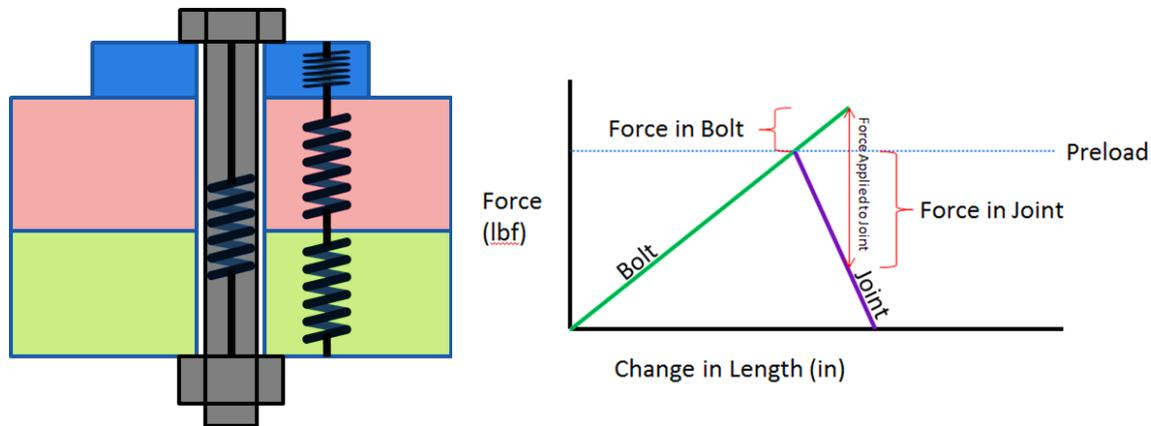
Fig. 1: Bolted joint modeled as a series of springs using Shigley's frustum of a cone approach
