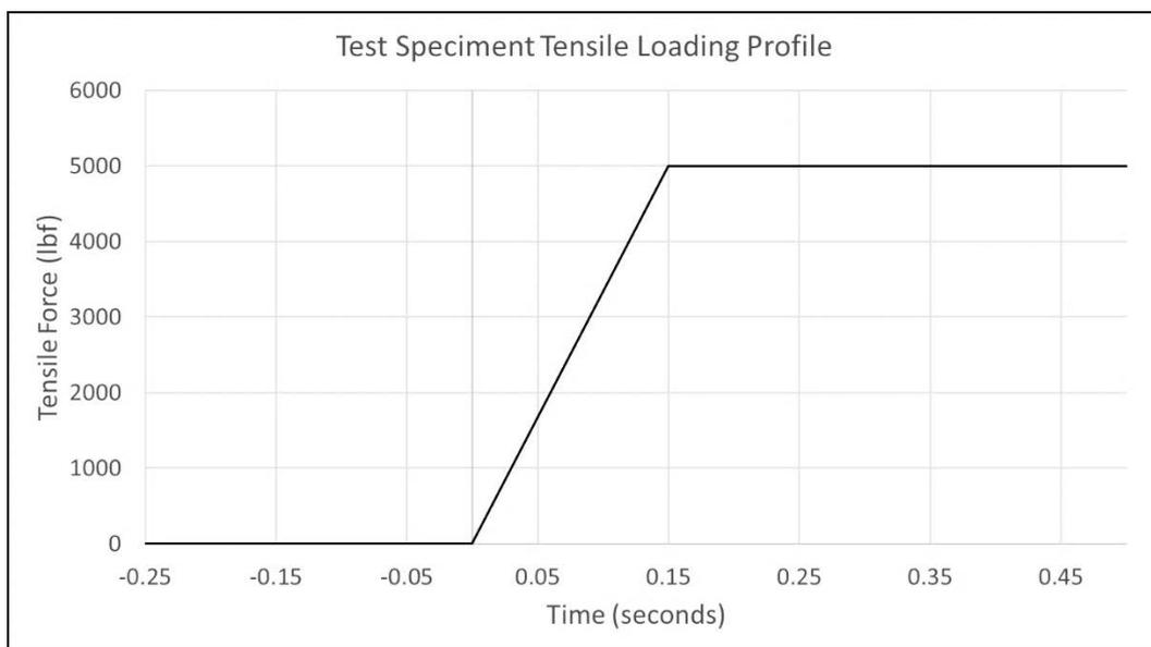
Fig.3: Tensile load profile of test specimen.
