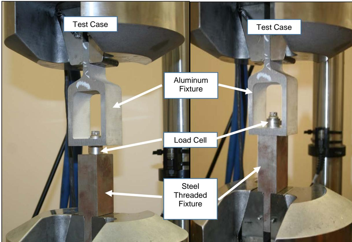
Fig.2: Test Setup A, depicted on the left, with the force transducer placed between the steel and aluminum plates and Test Setup B, depicted on the right, with the force transducer placed above the aluminum plate.
