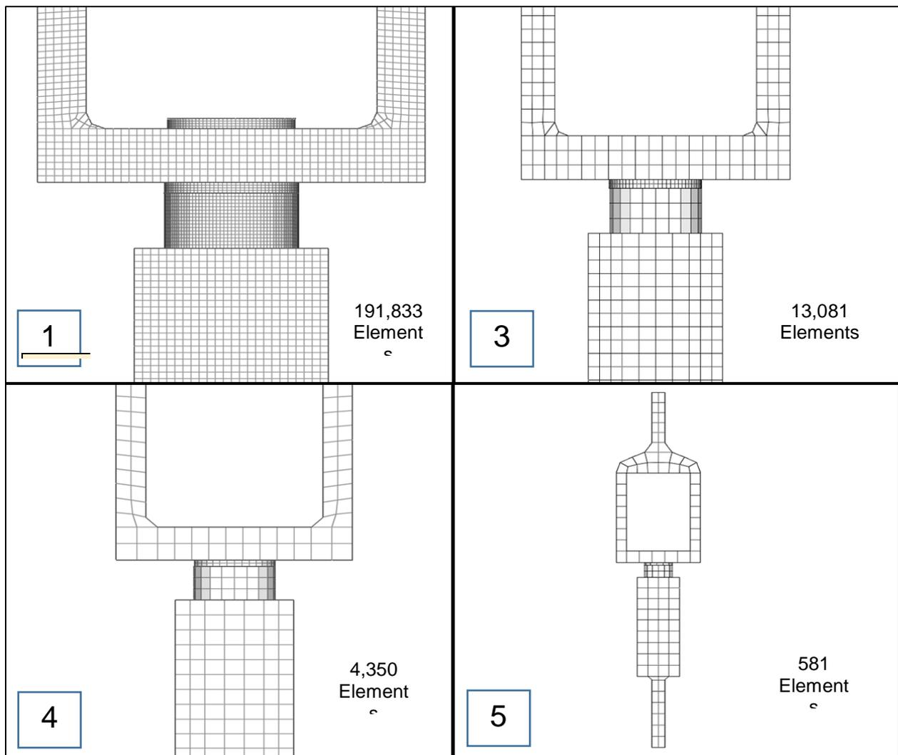
Fig.8: Depiction of various iterations in the mesh density of the test fixture in Test Case A. All of these iterations, with the exception of the bottom right (4), provided reasonably accurate results.
