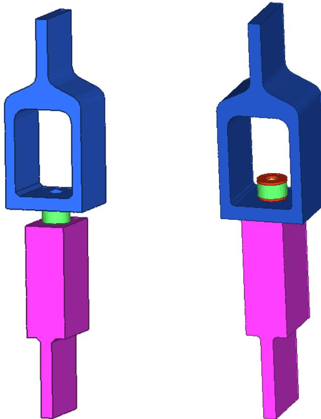
Fig.7: Finite Element Model, Test Case A depicted on the left and Test Case B depicted on the right.
