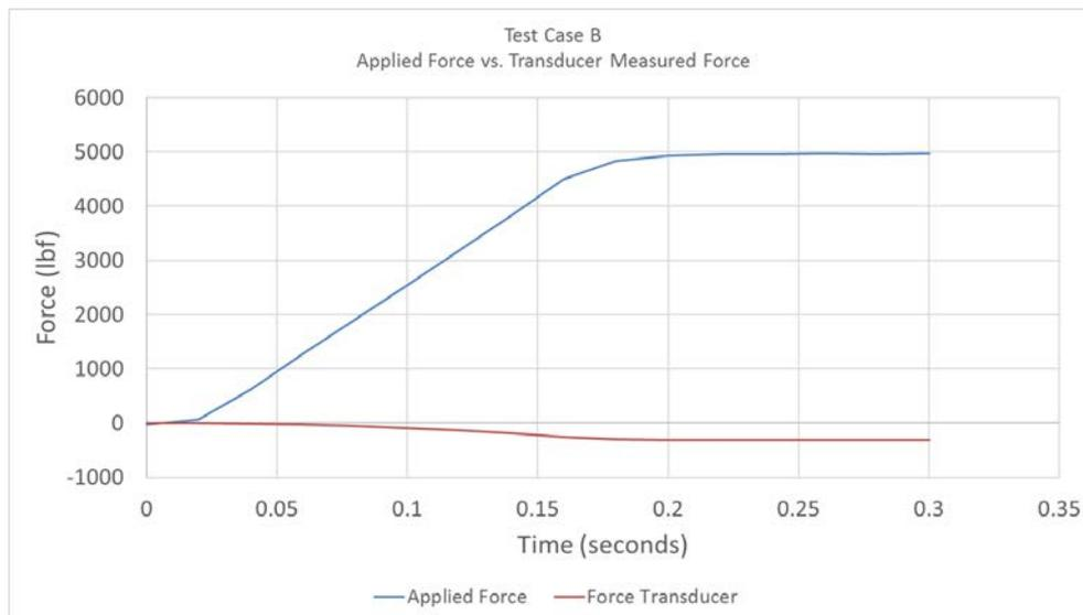
Fig.5: Graph of the applied force to the entire bolted joint and the load measured in the force transducer for Test Case B.
