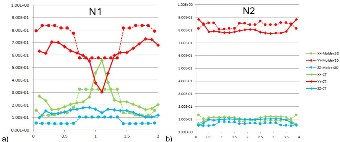
Fig.3: Degree of fibre orientation from microCT analyses and Moldex3D R14 injection molding simulations for the fibre-orientation specimens N1 and N2.
