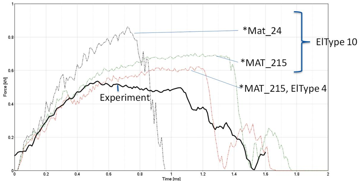
Fig.8: Force-time curves of the drop tower test on the component from experiment and simulation with different material models and element types.
