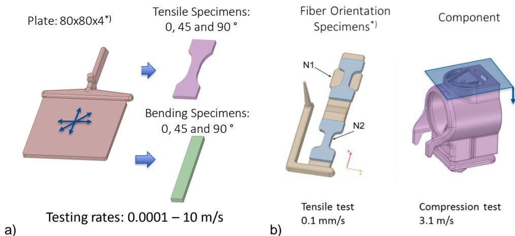
Fig. 1: Specimens and Testing for a) material characterisation and b) validation.
