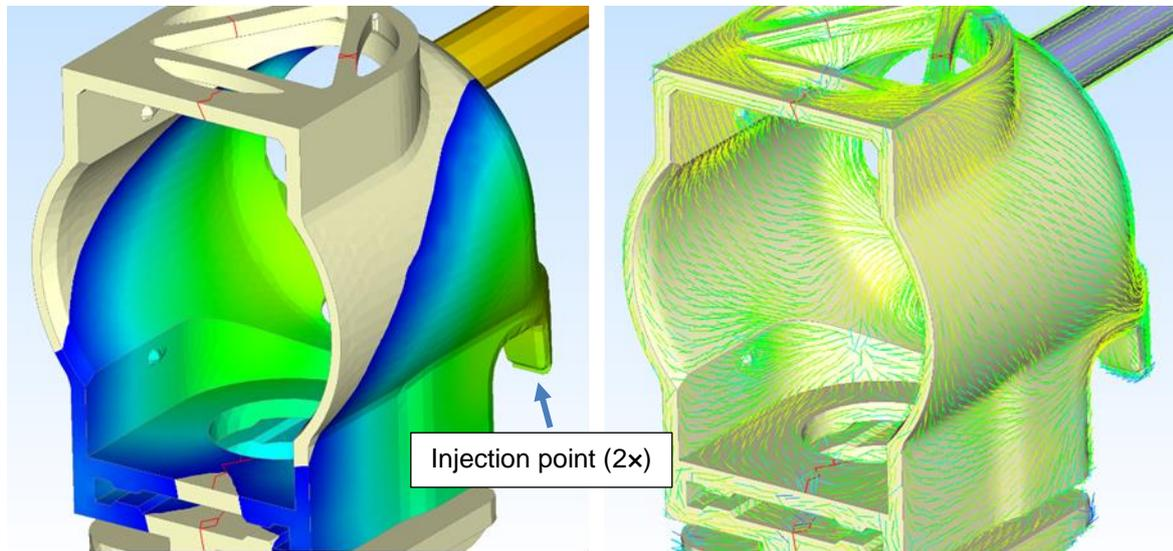
Fig.6: Pictures of the mould flow simulation results, showing the injection point, the melt front and the surface fibre orientation.
