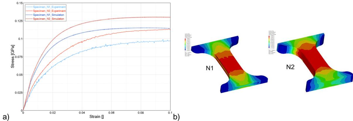
Fig.4: a) Stress–strain curves and b) simulated von-Mises stress fringe plots of fibre-orientation specimens during tensile testing. The formation of a mid-layer in specimen N1 leads to a reduced stress level in the core of the sample.
