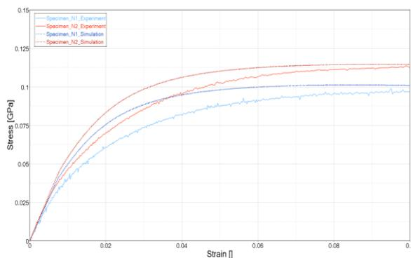
Fig.5: Stress-strain curves of the fibre-orientation specimens with simulated data with the modified material model accounting for the reduced fibre aspect ratio and the low strain rate.
