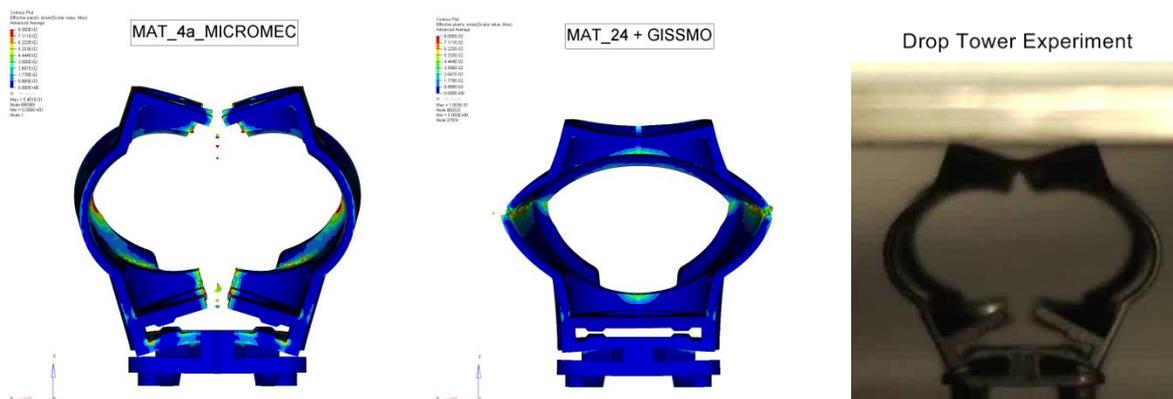
Fig.7: Failure mode of **\*MAT\_4a\_MICROMECH** model considering local anisotropies and isotropic **\*MAT\_024** Model in comparison with experimental drop tower experiment.
