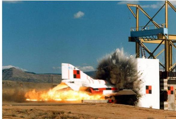
Fig.2: Dimensions of the target concrete block (left) and view of the impact (right) [5]
