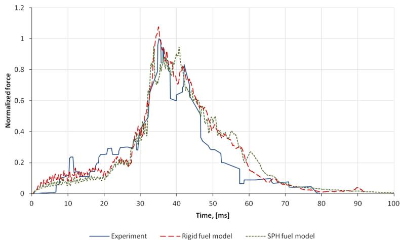
Fig.5: LTFs from analyses into rigid wall
