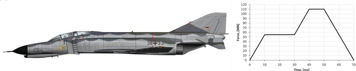
Fig. 1: McDonnell Douglas F-4 Phantom II (left) and its LTF (right)
