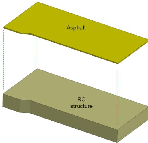
Fig.8: FE model of the target structure
