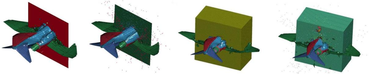
Fig.4: Impact of the FE airplane models into rigid wall and concrete block
