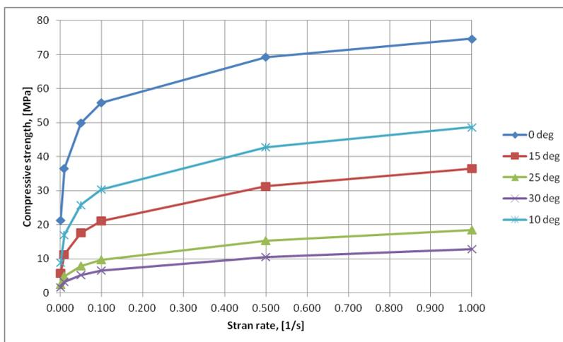
Fig.9: Asphalt compressive strength vs. strain rate
