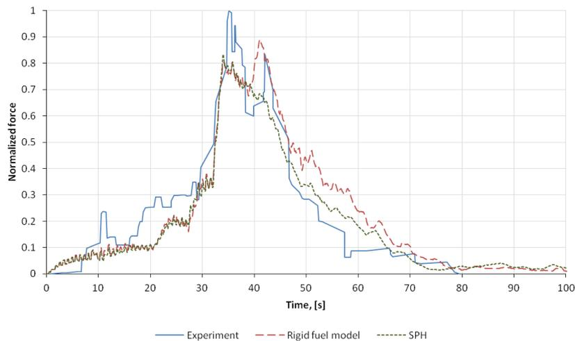
Fig.6: LTFs from analyses into concrete block
