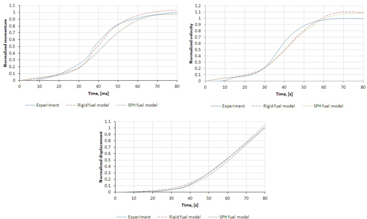
Fig.7: Normalized momentum, velocity and displacement of the concrete block
