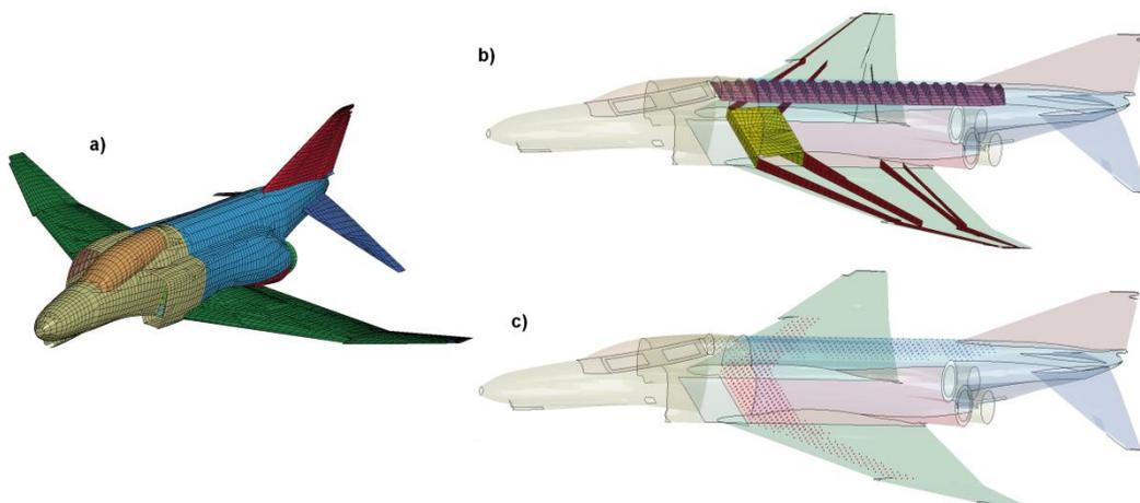
Fig.3: FE model of the airplane a), structural elements with lumped fuel mass b) and SPH fuel particles c)
