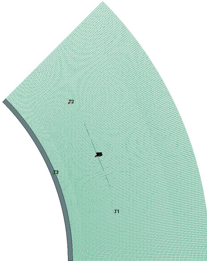
Figure 8 Illustration of 45 degree axisymmetric sector with target at zero angle of incidence and indicated location of tracer particles.
