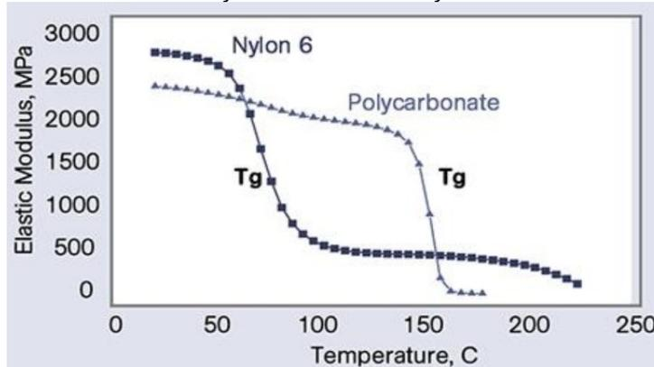
Fig.1: Modulus vs. temperature plot for unreinforced nylon 6 (semi-crystalline) and PC (amorphous). The material properties change significantly with the temperature and this will affect the mechanical response and consequently the flow around it.
