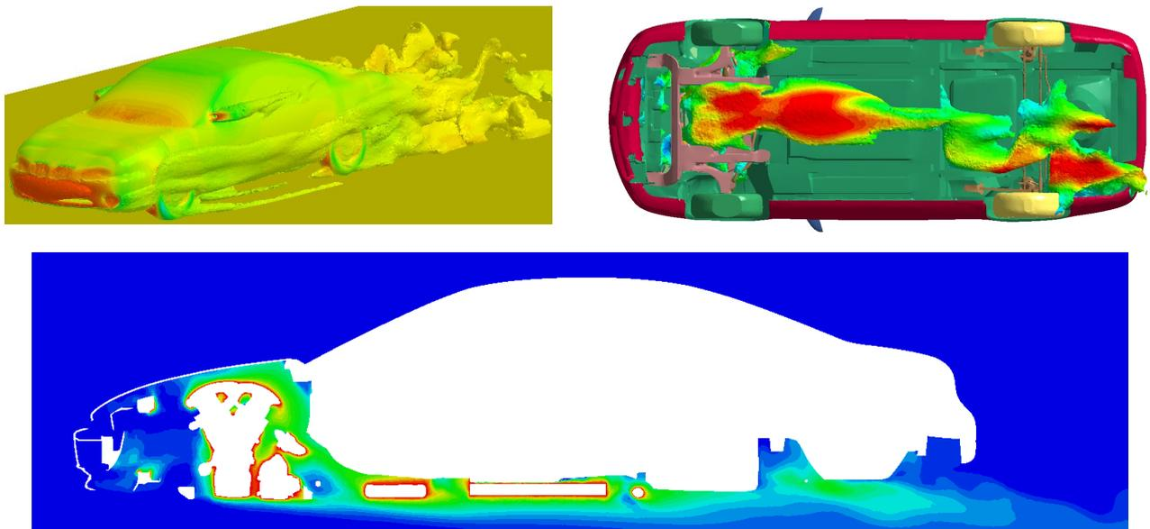
Fig.3: Results for the aerodynamics benchmark on a GMC vehicle. Top left shows the iso-surface of velocity, top right is iso-surface a fluid temperature and bottom is a cutplane with iso-contours of temperature showing the higher temperature around the engine block and exahust.
