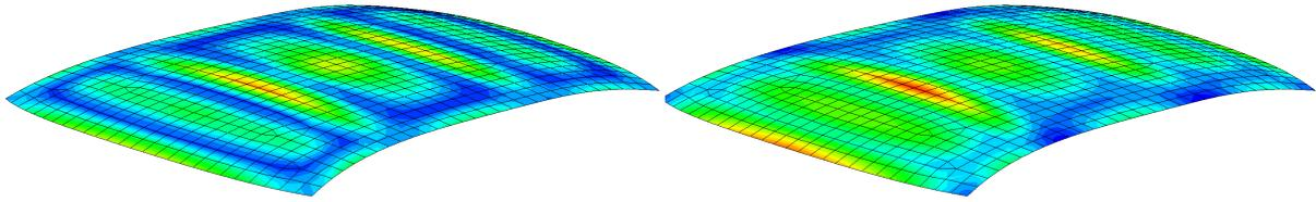
*Fig.5: From top to bottom: structural mesh on top of the CFD model for an FSI analysis of the roof pannel, post-processing of the flow around the vehicle using streamlines and structural displacement of the roof, Presure and structural stresses for the roo pannel.*
