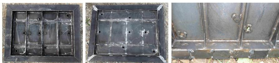
(a) front side (b) back side (c) spot welding in inserted plate
