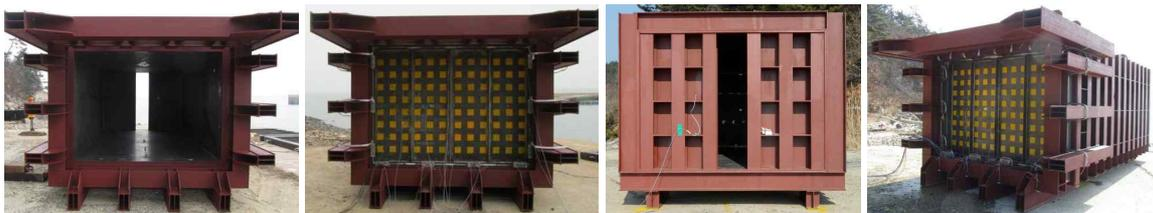
(a) front view without bulkhead (b) front view with bulkhead (c) rear view with opening (d) iso view of chamber test model
