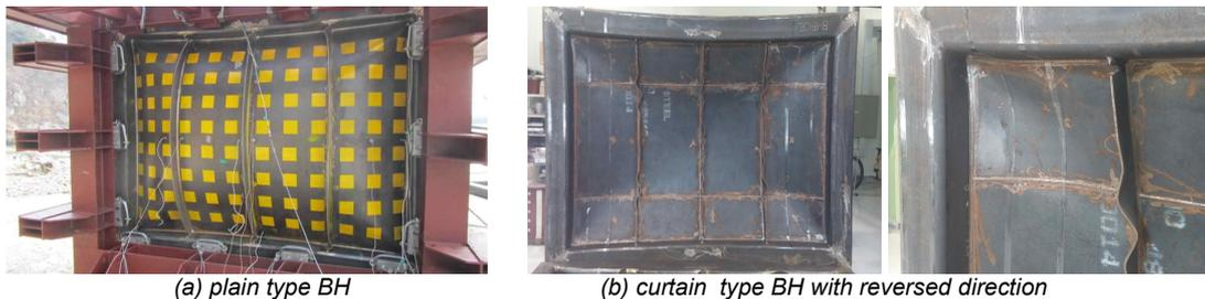
Fig. 9: Damage configuration of partial chamber bulkhead under internal blast test at  $1/2L$  stand-off distance
