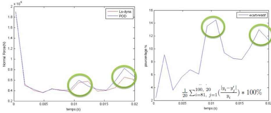
Fig.6: Typical time history of rigid wall force **reconstructed** at 14 time instances (arbitrary selection of one among 80 runs used for basis construction)
