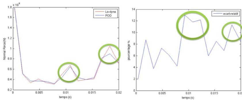
Fig.7: Typical time history of rigid wall force **predicted** at 14 time instances (arbitrary selection of one among 20 unused runs)
