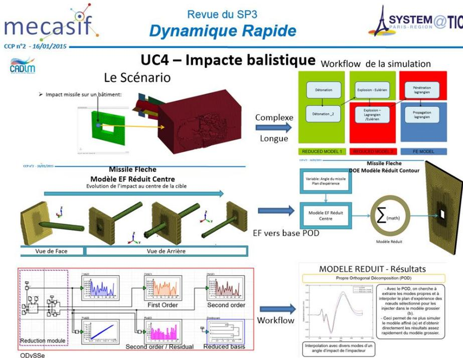
Fig.11: Application of POD method to ALE LS-DYNA for real-time (flight simulator) missile impact simulation conducted by CADLM for MECASIF project
