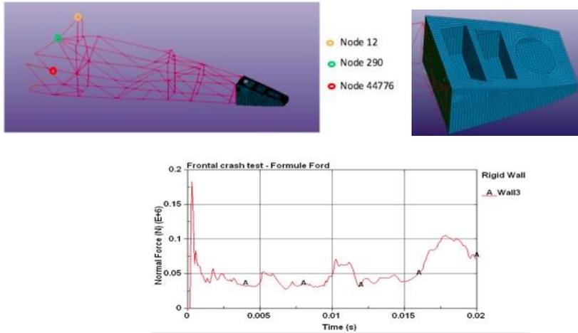
Fig.3: LS-DYNA simulations showing that the nose absorbs nearly 67% of the choc energy within 18 ms
