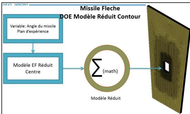
Fig.10: Missile impact zone replaced by its equivalent reduced model parametric studies reduced model to be used for parametric studies involving impact angle, velocity, mass, etc.
