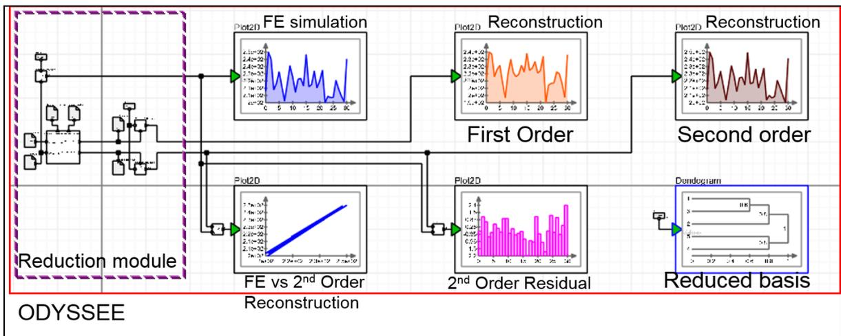
Fig.8: ODYSSEE Reduced Modelling Application for a 1<sup>st</sup> and 2<sup>nd</sup> order reconstruction of the response
