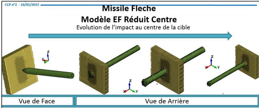
Fig.9: Missile impact zone with 10 Million elements
